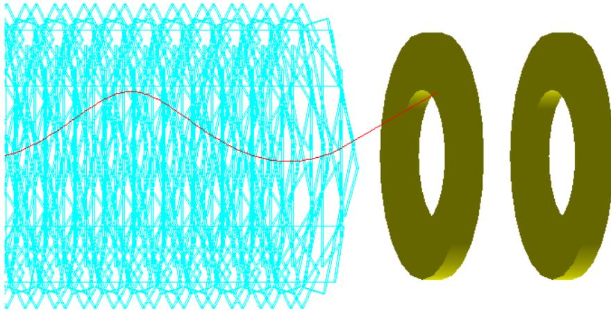
✓ The baseline design consists of two disks; each disk contains 930 hexagonal BaF<sub>2</sub> crystals
