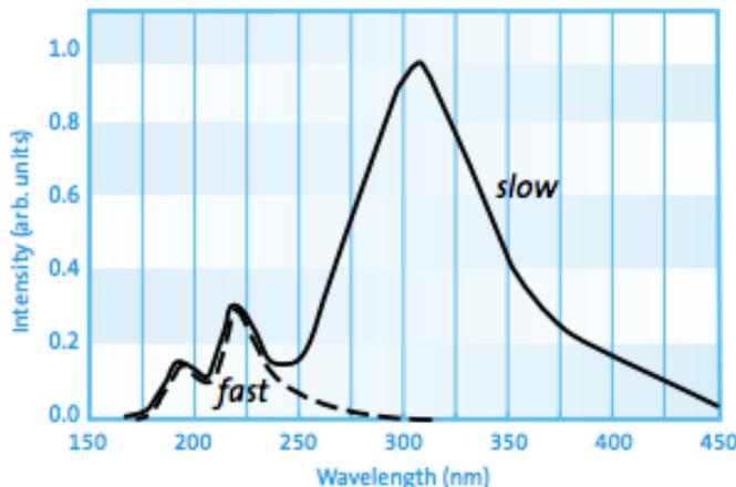
Figure 1. Scintillation emission spectrum of BaF<sub>2</sub>
