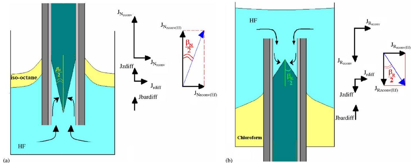
Fig. 2. Schematic diagram of the experiment for TE (a) and for RTE (b). The vectorial diagrams describe the fluxes in the two experimental geometries.
