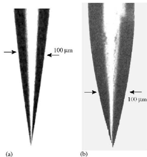
Fig. 1. Optical images of SNOM probes produced by TE (a) and by RTE (b) in the same experimental conditions.
