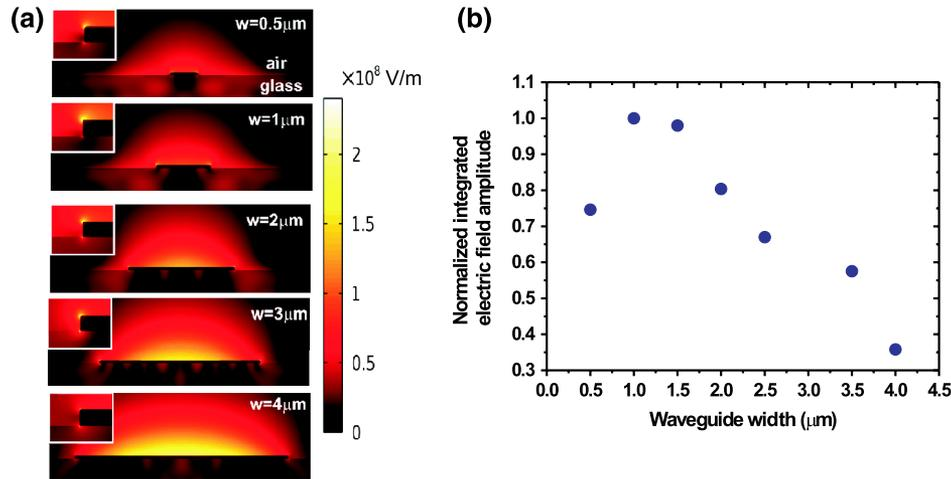
Fig. 4. (Color online) (a) Computed lateral distributions of the surface plasmon electric field for different widths  $w$  of Au stripe.  $\lambda = 800$  nm, Au thickness = 50 nm. The insets display a magnified area around the left-hand-side corner. The high field magnitude located at the corner is readily visible. (b) Normalized electric field magnitude integrated in a  $27 \text{ nm} \times 27 \text{ nm}$  area around the corners as a function of waveguide width.
