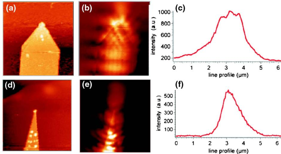
Fig. 6. (Color online) Near-field images of selected waveguides and tapers. (a) Topography of a  $3.5 \mu\text{m}$  wide stripe terminated by a  $70^\circ$  taper, (b) corresponding near-field optical map, and (c) optical profile taken at the end of the taper in (b); (d) topography of a  $3.5 \mu\text{m}$  wide stripe terminated by a  $20^\circ$  taper, (e) corresponding near-field optical map, and (f) optical profile taken at the end of the taper in (e).
