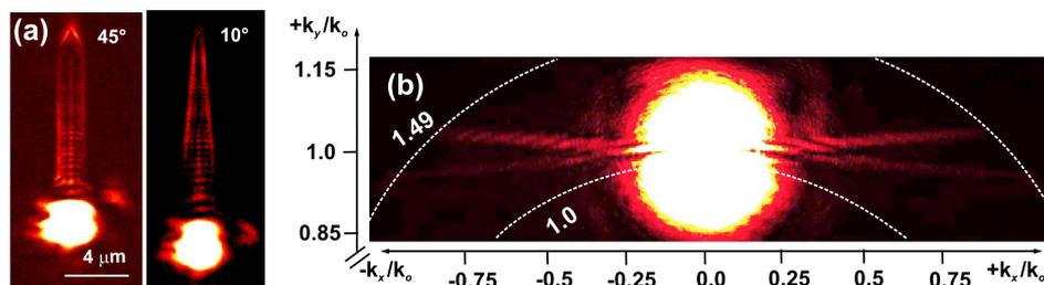
Fig. 5. (Color online) (a) Leakage images of a surface plasmon propagating in an Au stripe ( $w = 2 \mu\text{m}$ ), terminated by a taper with an opening angle  $\theta$  of  $45^\circ$  (left image) and  $10^\circ$  (right image), (b) corresponding partial Fourier plane  $\theta = 10^\circ$ . Note the two inclined lines, the signature of diffraction at the edges of the taper.
