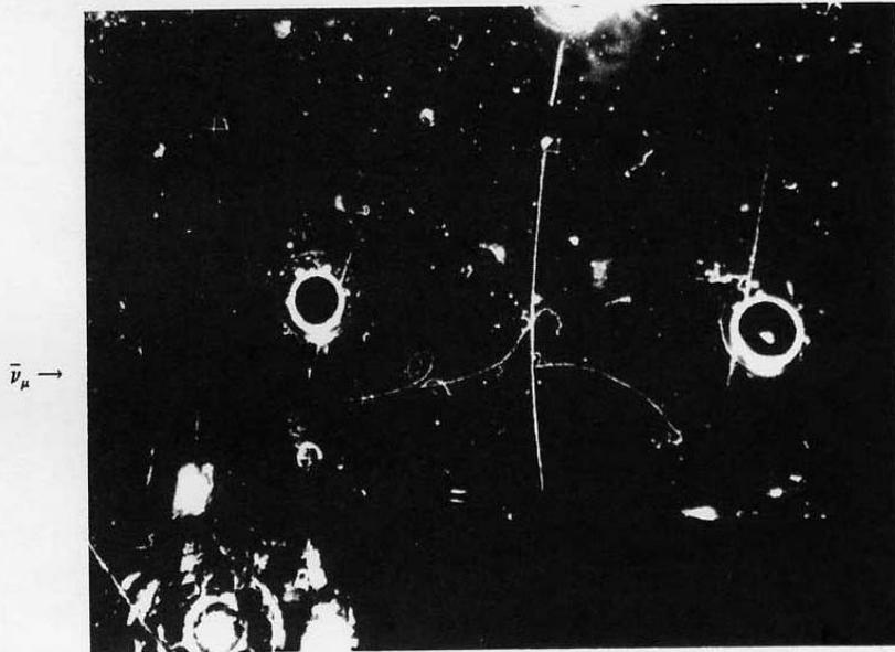
**Figure 10.6** The first picture of a neutral weak process ( $\bar{\nu}_\mu + e^- \rightarrow \bar{\nu}_\mu + e^-$ ). The neutrino enters from the left (leaving no track), and strikes an electron, which moves off horizontally to the right, emitting two photons (which show up in the picture only when they subsequently produce electron-positron pairs) as it slows down and spirals inward in the superimposed magnetic field. (Photo courtesy CERN.)
