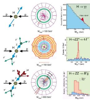
Higgs to 2 photons (M<sub>u</sub> < 140 GeV) .  $H^0 \rightarrow \gamma \gamma$  is the most promising channel if  $M_{\omega}$  is in the range 80 - 140 GeV. The high performance PbWO, crystal electromagnetic calorimeter in CMS has been optimized for this search. The  $\gamma\gamma$  mass resolution at M $\gamma\gamma \sim 100$  GeV is better than 1%, resulting in a S/B of  $\approx 1/20$
