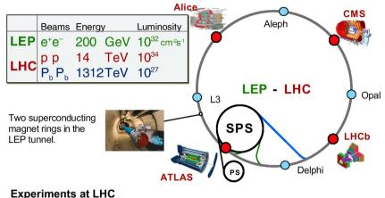
ATLAS A Toroidal LHC ApparatuS. (Study of Proton-Proton collisions) CMS Compact Muon Solenoid. (Study of Proton-Proton collisions) ALICE A Large Ion Collider Experiment. (Study of Ion-Ion collisions) LHCb (Study of CP violation in B-meson decays at the LHC collider)
