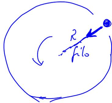
$$\begin{aligned}\vec{a}(t) &= -\omega^2 \vec{r}(t) = \frac{d^2 \vec{r}(t)}{dt^2} = \left( \frac{d^2 x}{dt^2}, \frac{d^2 y}{dt^2} \right) \\ &= -\omega^2 (x, y)\end{aligned}$$
