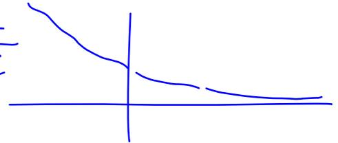
$$I(t) = \frac{dQ}{dt} = \frac{d}{dt} \left( Q_0 e^{-\frac{t}{RC}} \right) =$$
