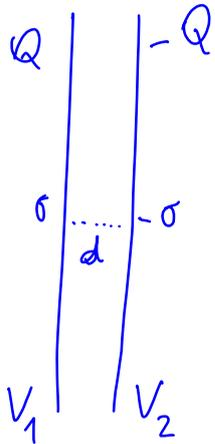
$$\sigma = \frac{Q}{A} \quad A = \text{superficie armatura}$$
