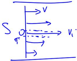
$$Q = \sum_i \sigma_i v_i = S v_{medza}$$
