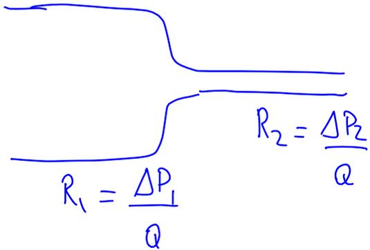
$$R_{\text{tot}} = R_1 + R_2$$
