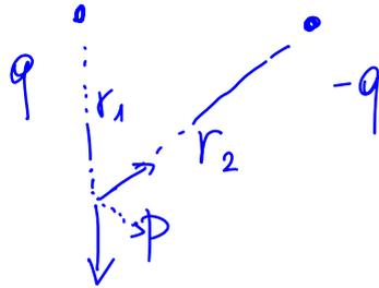
$$V(r_1, r_2) = k \frac{q}{r_1} + k \frac{-q}{r_2}$$
