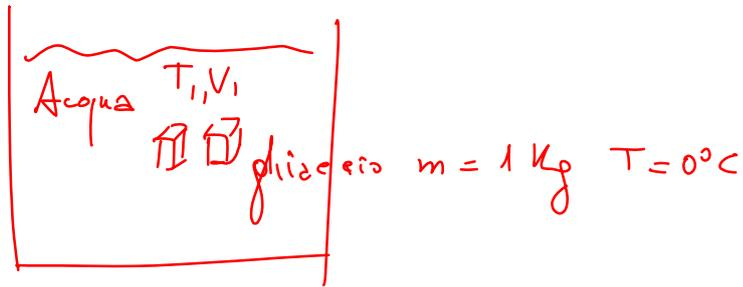
$$Q_{\text{fusione}} = k_{\text{m ghiaccio}} = \frac{80 \text{ cal}}{\text{gr}} 10^3 \text{ gr} = 80 \text{ kcal}$$
