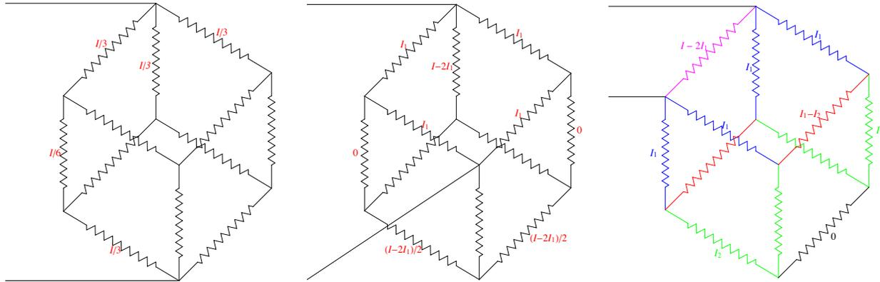
Figura 10.1: (a), (b), (c) : circuito a cubo..
