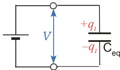
$$q_1 = C_1 V; \quad q_2 = C_2 V; \quad q_3 = C_3 V$$
