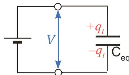
$$\frac{1}{C_{eq}} = \frac{1}{C_1} + \frac{1}{C_2} + \frac{1}{C_3}$$
