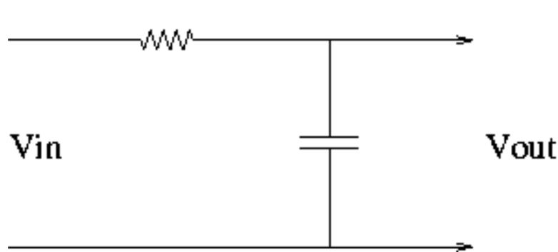
$$\frac{q}{C} + R \frac{dq}{dt} = V_{in}, \quad V_{out} = V_C = \frac{q}{C}$$
