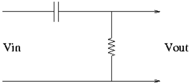
$$\frac{q}{C} + R \frac{dq}{dt} = V_{in}, \quad V_{out} = V_R = Ri$$
