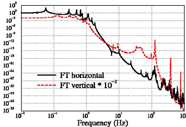
Figure H.2: The Virgo superattenuator performance: transfer functions (TF) predicted by the simulation for the attenuation of vertical and horizontal motions.
