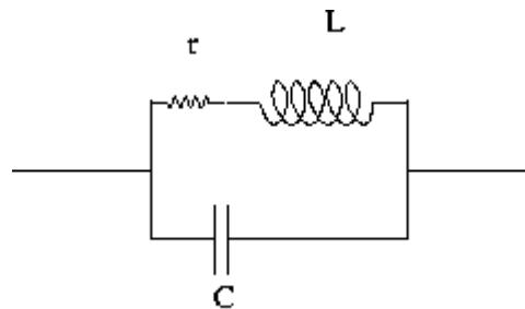
$$Z = \frac{Z_L Z_C}{Z_L + Z_C} = \frac{(r + j\omega L)/(j\omega C)}{r + j\omega L + 1/j\omega C} = \frac{r + j\omega L}{j\omega r C - \omega^2 LC + 1}$$
