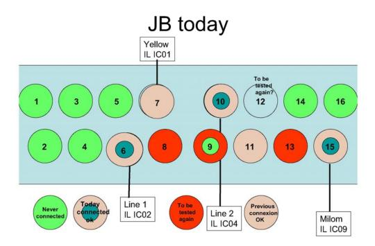
Apparently, out of the 16 connectors, one (nr 6) is used for the Line1, one (nr 15) is used for the Milom, one (nr 10) is ready for Line 2, three (8, 12 and 13) are not working. Two of these (nr 8 and nr 13) are to be tested again. IL IC01 is connected to connector nr 7.
