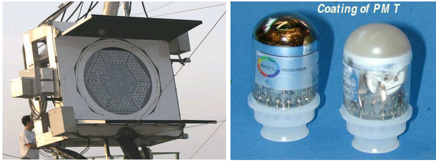
Figure 2. On the left a view of the telescope camera with its 577 PMTs. The inner section of the camera is made up of 397 0.1^\circ field-of-view pixels, surrounded by four rings of 0.2^\circ pixels. The second picture shows two Electron Tubes PMTs. The “frosted” PMT on the right has been coated with a wavelength shifter lacquer that increases the quantum efficiency by 30% (coating all the PMTs is roughly equivalent to increasing the mirror area from 240 \text{ m}^2 to 300 \text{ m}^2 .)
