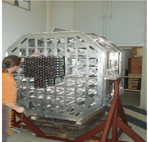
Fig. 25. The first H.E.S.S. camera frame at the University VI – VII in Paris, in spring 2001 (with J.-P. Tavernet standing in front). At this stage the camera was partly equipped with photomultipliers and the corresponding electronics in the back. In full configuration the camera has a total number of 980 phototubes (pixels) and a weight of about 860 kg.
