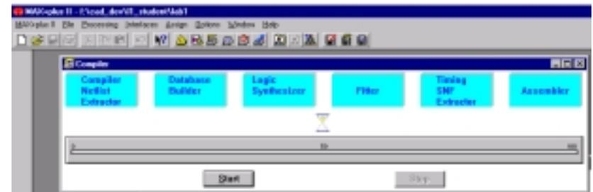
After creating schematic or VHDL file, clicking on start button will start compilation process. After compilation is complete, can simulate design (if you have created a test waveform for the design).
