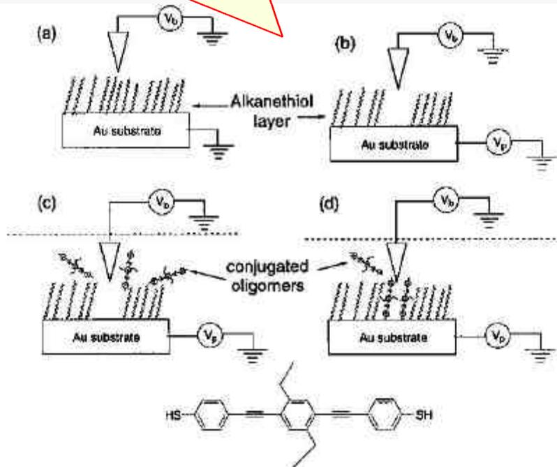
Figure 4.6 Schematic representation of the lithographic patterning and replacement of conjugated molecules in an alkanethiolate matrix. (a) Normal STM imaging of an alkanethiolate SAM with tip bias  $V_b$ . (b) SAM removal by applying a voltage pulse  $V_p$  to the substrate. (c) Carrying out the same voltage pulse as in (b), but under a solution of molecular wires (expanded structure at bottom) causes (d) insertion of the wires into the newly vacated site.
