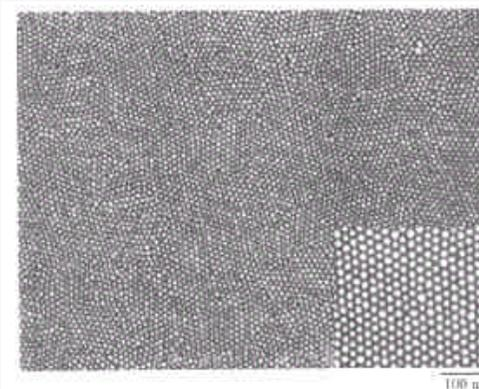
Figure 1. Scanning electron micrograph of a LB monolayer consisting of dodecanethiol-encapsulated gold nanoparticles of 8.3 nm in diameter, displaying long range order [18]. The inset shows higher magnification which reveals hexagonal close-packed structure.
