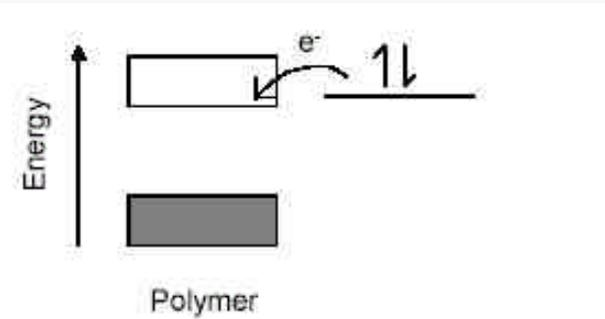
Reducing agents such as calcium and lithium can introduce electrons into the conduction band of a conjugated polymer.
