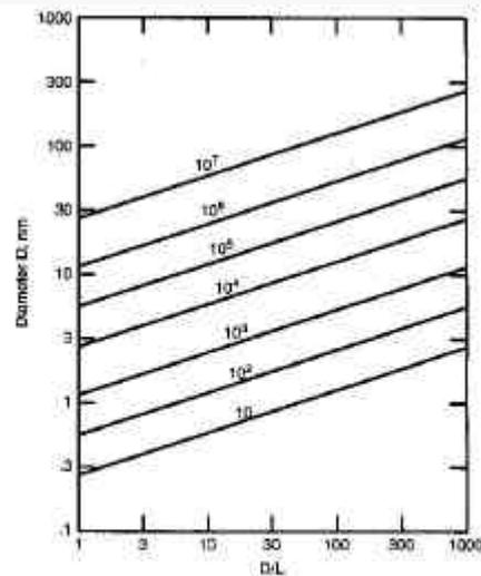
Figure 11.2. Dependence of the diameter  $D$  of a cylindrical polymer on its diameter: length ratio  $D/L$  for molecular weights from 10 to  $10^6$  Da, as indicated on the curves. A density  $\rho = 1 \text{ g/cm}^3$  was assumed in Eq. (11.13) for plotting these curves.
