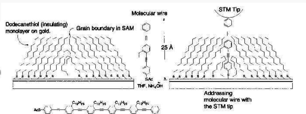
Figure 4.3 Protocol for inserting molecular wires into dodecanethiolate SAMs at grain boundaries and step edges. Relative conductance recording was done with a STM tip. The molecule at the bottom has also been used in this study.
