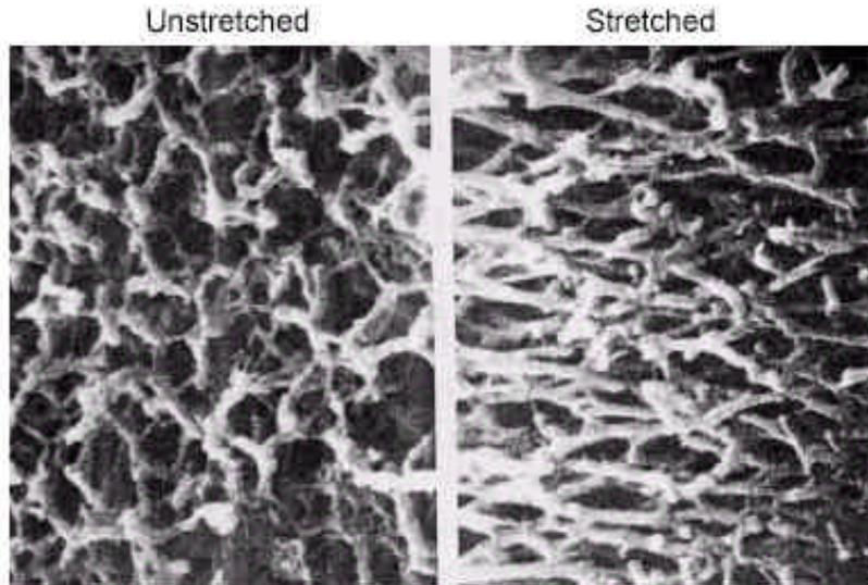
Stretching polyacetylene aligns the chains and improves conductivity. Each fiber shown here consists of about 1,500 polymer chains. A goal of molecular electronics is to use individual polymer chains.
