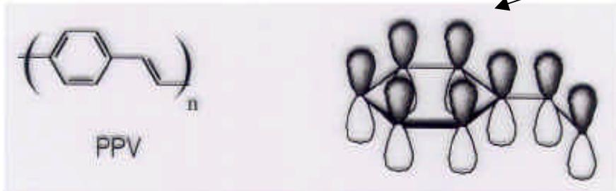
Each p electron in the unit cell results in one  $\pi$  band.
