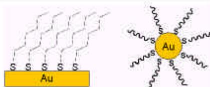
Figure 6. Schematic illustration of SAM (left) and MFCs (right) of alkanethiol molecules on gold substrate and nanoparticle.
