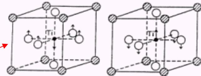
Perovskite ceramics with large static dielectric constant ( $\sim 200$ ) and negligible ferroelectricity
