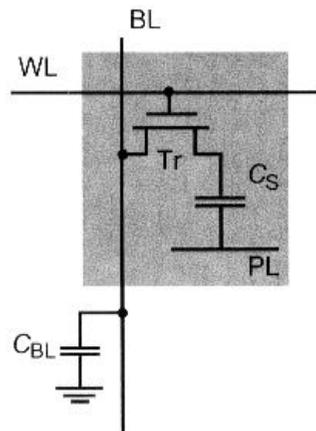
Figure 2: Schematic representation of a DRAM memory cell.
