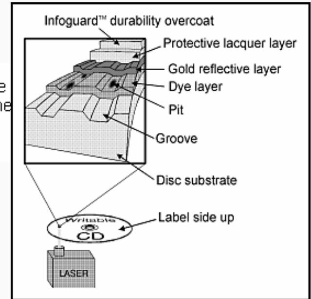
Grooves are frequently scribed on the substrate to enhance optical absorption, so favoring writing
