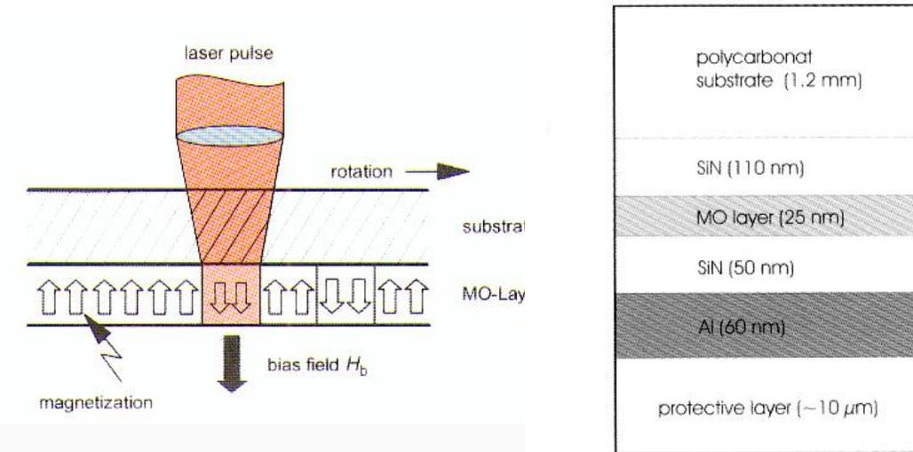
Figure 4: Layer stack of a typical MO disc [2].
