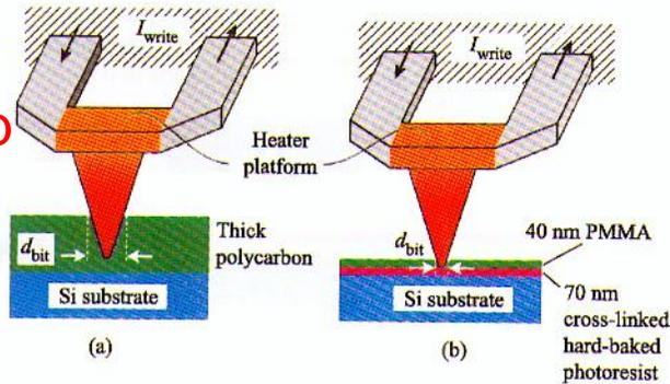
**Figure 2:** (a) Earlier storage medium consisting of a bulk polycarbonate layer. (b) New storage medium for smaller bit sizes, consisting of a thin writable PMMA layer on top of Si substrate separated by a cross-linked film of photoresist. From [13], reproduced with permission.
