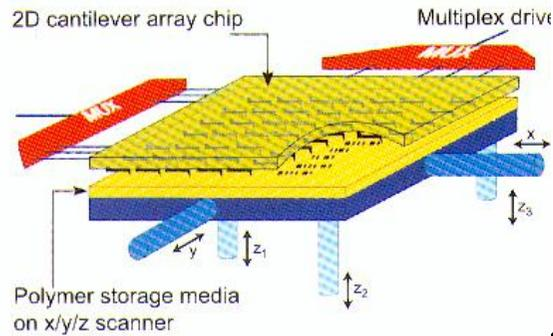
**Figure 1:** “Millipede” concept. Reproduced with permission from [23](a), © 1999 IEEE.
