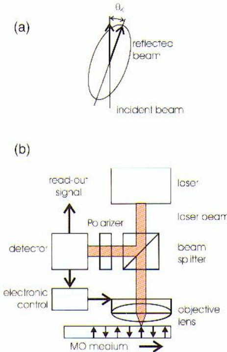
Figure 2: Read-out by the magneto-optical Kerr effect (MOKE).
