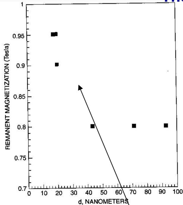
Figure 7.5. Dependence of the remnant magnetization  $M_r$  on the particle size  $d$  of the grains that form the structure of a Nd-B-Fe permanent magnet normalized to the value  $M_s$  (for a 90-nm grain size). [Adapted from A. Manaf et al., *J. Magn. Magn. Mater.*, **101**, 360 (1992)]
