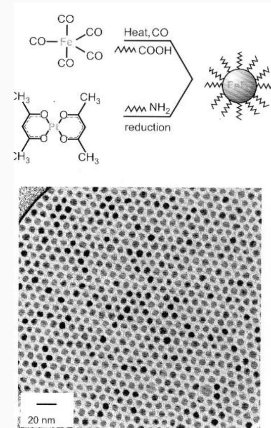
Figure 24: TEM micrograph of self assembled FePt nanoparticles (bottom). The schematic illustrates the fabrication roots for this self-assembled material (top) [19].
