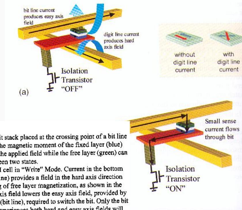
**Figure 2:** TMR bit stack placed at the crossing point of a bit line and a digit line. The magnetic moment of the fixed layer (blue) does not move in the applied field while the free layer (green) can be switched between two states.
