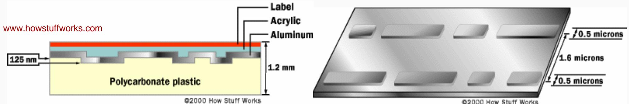
CD-ROM (original design): bits are “holes” impressed in a reflecting Al film evaporated onto a polycarbonate substrate
