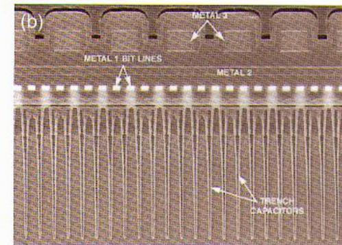
Figure 3: Example of a 3-D capacitor: (cross section) deep trench with oxide/nitride dielectric ( $\epsilon_r \approx 7$ ). (a) Schematic, from [8]; (b) Scanning electron micrograph for Toshiba/Infineon 64 Mb chip. The design is similar in 256 Mb and 1 Gb chips with much higher aspect ratios (height/depth).
