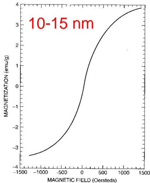
Figure 7.4. Reversible magnetization curve for nanosized powders of a Ni-Fe-Co alloy that exhibits no hysteresis. An oersted corresponds to  $10^{-4}$  T (tesla). [Adapted from K. Shafi et al., *Mater. Res.* 15, 332 (2000).]
