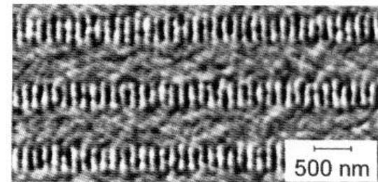
Figure 1: Magnetic force micrograph (MFM) of recorded bit patterns. Track width is 350 nm. The tracks are written at a frequency (linear bit density) slightly lower than used in the actual HDDs and every second track is skipped in order to give a clearer image.
