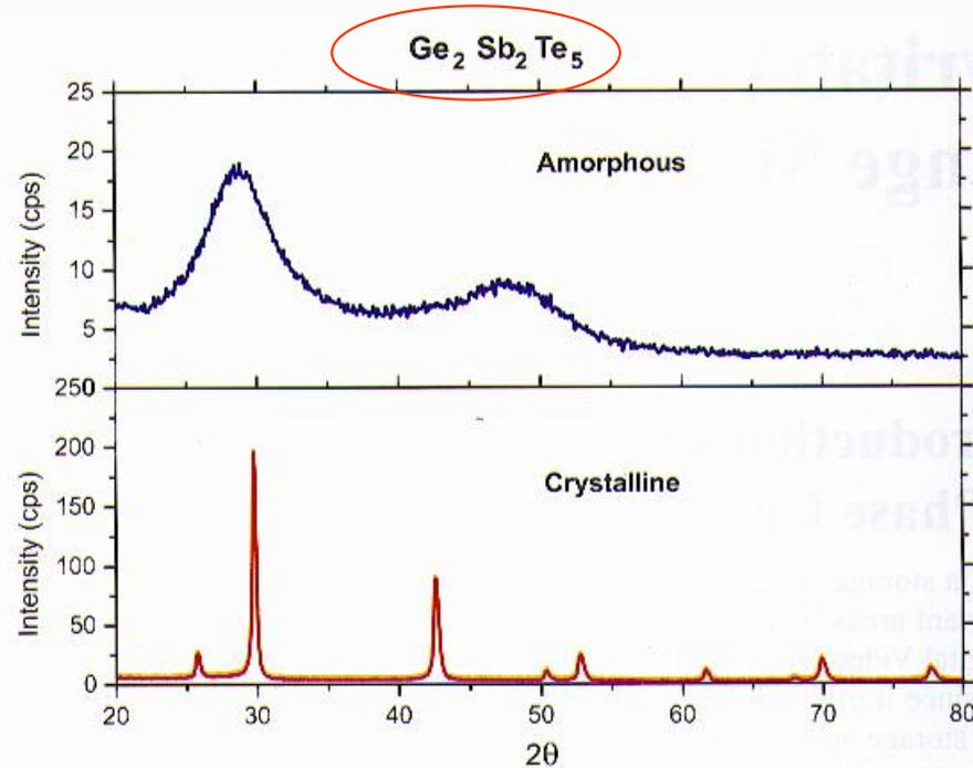
**Figure 2:** x-ray diffraction spectrum of a thin film of phase change material ( $\text{Ge}_2\text{Sb}_2\text{Te}_5$ ) after deposition (amorphous) and after heating to  $200^\circ\text{C}$  (crystalline).
