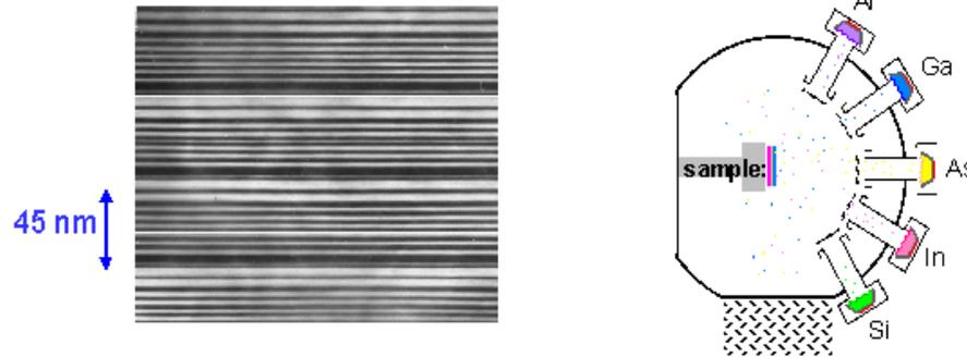
Cross-section of a few stages of QC-laser crystal crystal growth one atomic layer at a time
