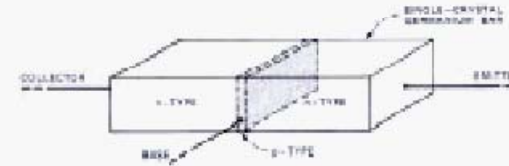
Figure 1 – The first transistors: (a) the point contact transistor of Brattain and Bardeen, 1947 (left); (b) the junction transistor of Shockley, Morgan, Sparks, and Teal, 1950 (right).
