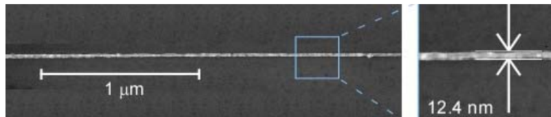
Ti/Al gate structures for a SET device generated by e-beam lithograph and lift-off.
