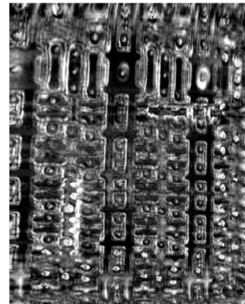
g. 2. Topography (left) and oblique reflection (right) micrographs of aluminum structures buried underneath interlayer dielectrics.
