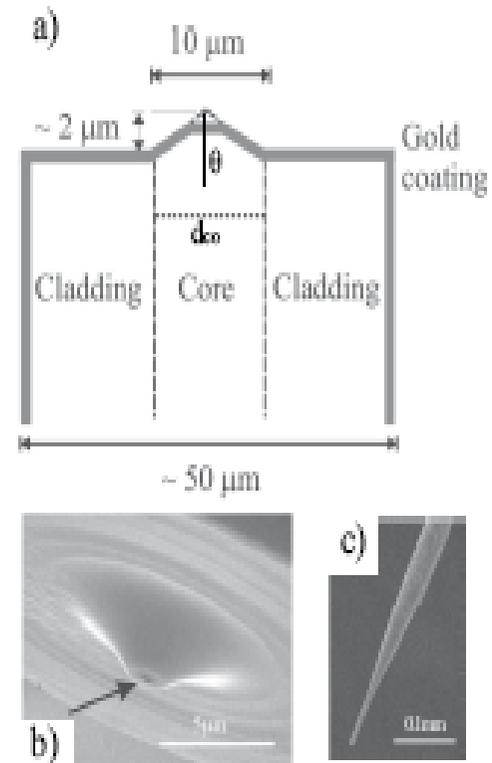
The final result is a conical (tapered) optical fiber, with the taper metal-coated in order to prevent losses, and an apical (uncoated) hole playing the role of the aperture
