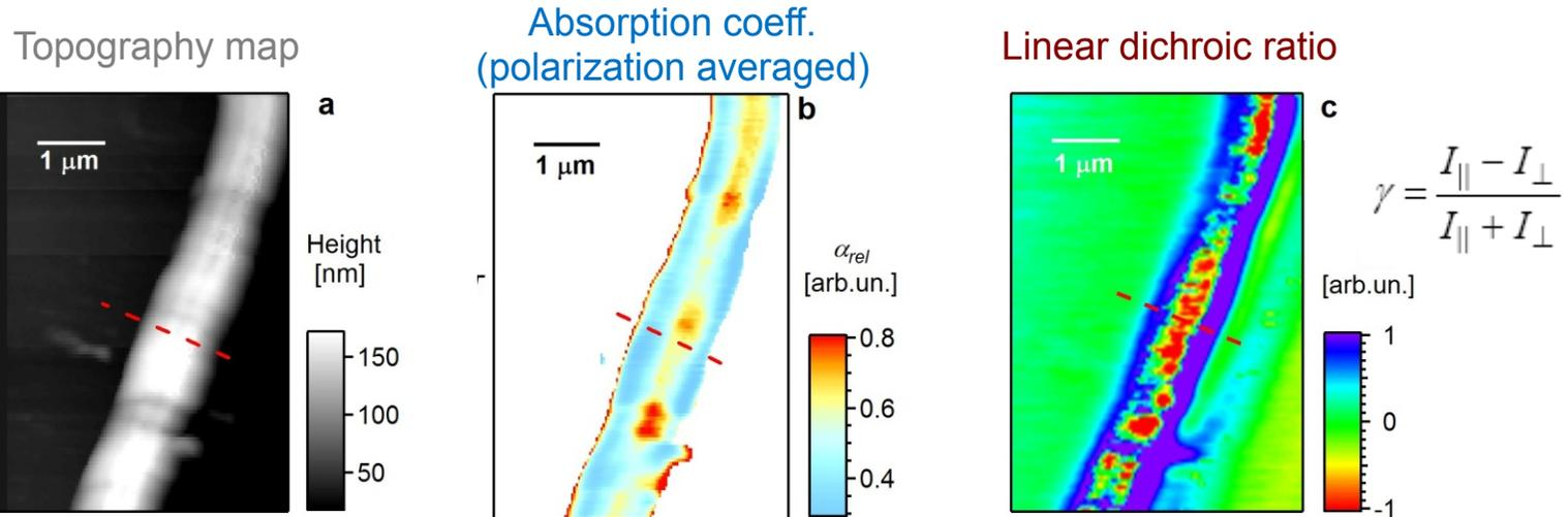
Line profiles of topography, absorption, dichroic ratio
