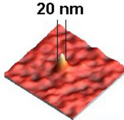
SNOM image of a single dye molecule anchored on a substrate
