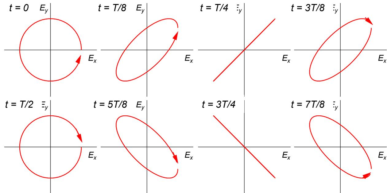
At the SNOM probe input, laser polarization is periodically manipulated (circular-elliptical-linear)
