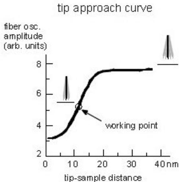
If the tip is kept in **longitudinal** oscillation, the oscillation amplitude depends on the distance due to shear-forces (mostly associated with friction of the air layers between tip and surface)
