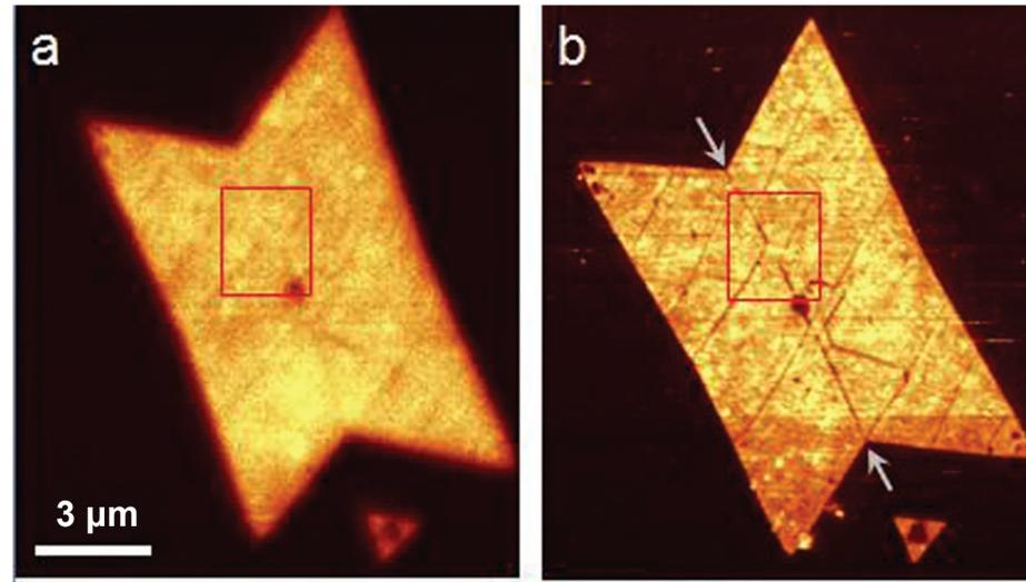
SNOM and confocal PL images of butterfly-shaped monolayered MoS<sub>2</sub> prepared on an ITO-coated glass substrate
