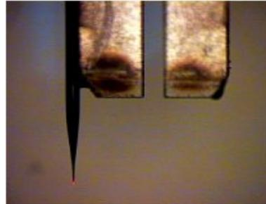
Fiber tip is glued onto a *tuning fork* (a quartz diapason acting as a mechanical oscillator and showing capabilities to measure the oscillation amplitude)
