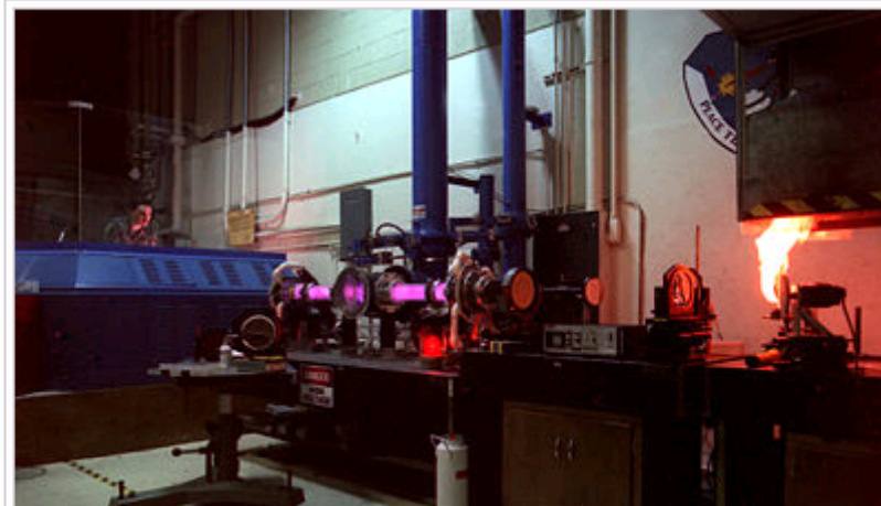
A test target is vaporized and bursts into flame upon irradiation by a high power continuous wave carbon dioxide laser emitting tens of kilowatts of infrared light.
