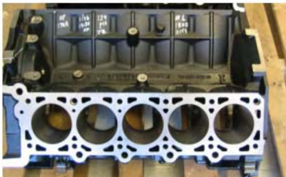
Fig. 5. A picture of the engine showing the cylinder deck face to be measured for flatness
