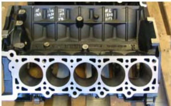
Fig. 5. A picture of the engine showing the cylinder deck face to be measured for flatness
