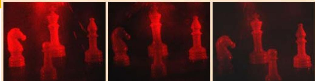
These three images of the same hologram were taken by positioning the camera at three positions, moving from left to right. Note that the pawn appears on the left side of the king in the left photo, but transitions to the right of the king as you sweep your eye across the hologram. This is real parallax, which tells you that the image is truly 3-dimensional. Each perspective corresponds to looking through the hologram at a particular point.
