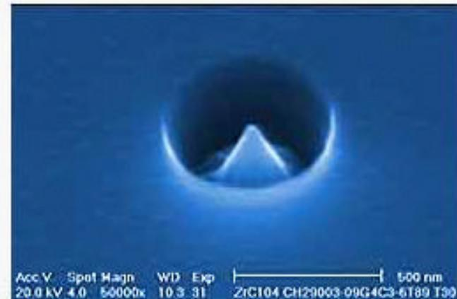
This carbide crystalline tip, with a radius of 100 angstroms, or 10 nanometers at the top and 0.5 micron at the base, emits electrons in a tiny beam.
