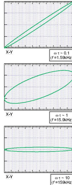
FIG. 4. Same of Fig. 3, but simulating the oscilloscope in the X-Y operating mode (Y is channel 2, X is channel 1). The same V/DIV setting is used for all plots (for both channels).
