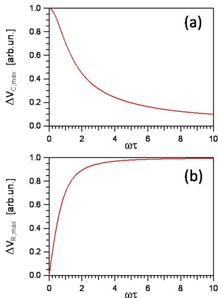
FIG. 2. Numerical calculations of the maximum amplitude  $\Delta V_{C,max}$  and  $\Delta V_{R,max}$  defined in the text [plot (a) and (b), respectively] as a function of  $\omega\tau$ . Bear in mind that  $\omega = 2\pi f$ , with  $f$  frequency of the alternate generator. High and low frequencies components of the "input" signal  $V(t)$  are practically cut (heavily suppressed) depending on whether the "output" signal is measured across the capacitor or the resistor.
