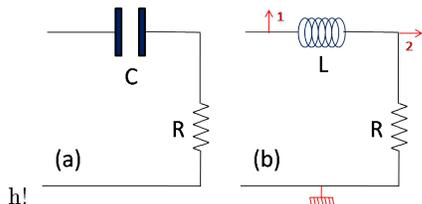
FIG. 1. Schemes of the simple circuits considered in the text, made of a resistor-capacitor (a) and resistor-inductance series (b).
