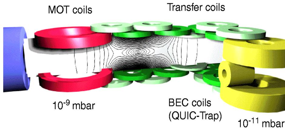
Figure 1: Experimental setup for the magnetic transfer of atoms.
