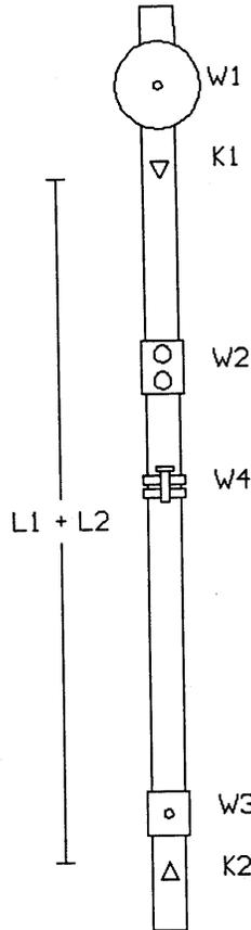
Figure 1: Diagram of the Kater pendulum. The symbols  $L_1$  and  $L_2$  on the figure are  $\ell_1$  and  $\ell_2$  in the text.  $L = \ell_1 + \ell_2$  is the distance between fulcrum points. The distances of most of the weights from each fulcrum are adjustable. Note that W2 is between W4 and W3, rather than as shown.
