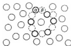
FIG. 1. Typical configuration of the atoms. If an excitation represents rotation of a ring of atoms such as the six in heavy outline the wave function must be plus if they are in the \alpha positions and minus if they are moved to the intermediate \beta positions.
