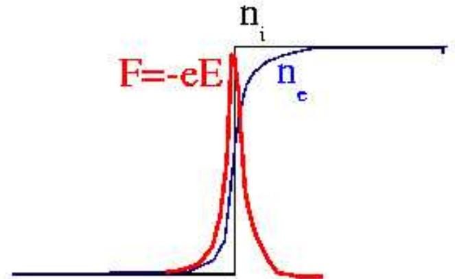
In an external field  $E_d$ , electrons are reflected from the sheath if  $v_{osc} = eE_d/m_e\omega < v_{th}$ .
