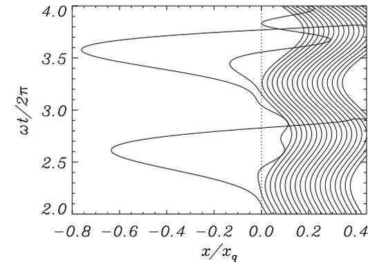
An **irregular aperiodic motion** is observed with electrons re-entering the plasma with energy  $\approx$  **the oscillation energy in vacuum**.
