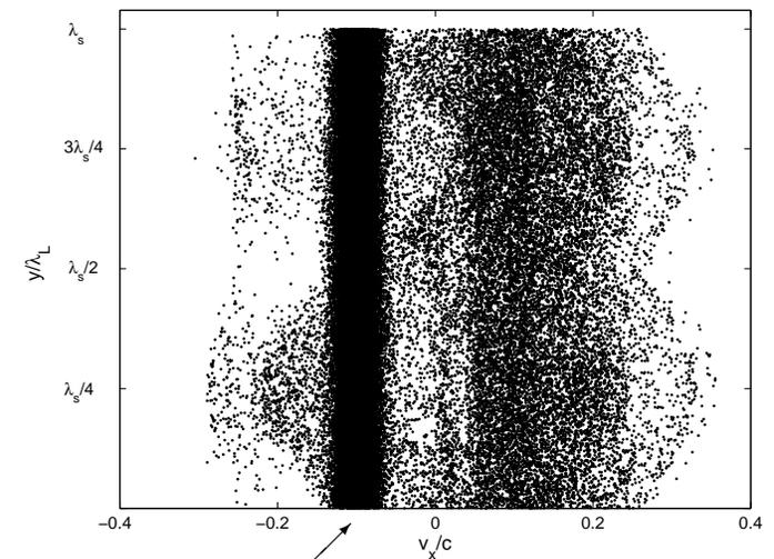
PIC and test-particle simulations both show enhanced electron heating near SW maxima
