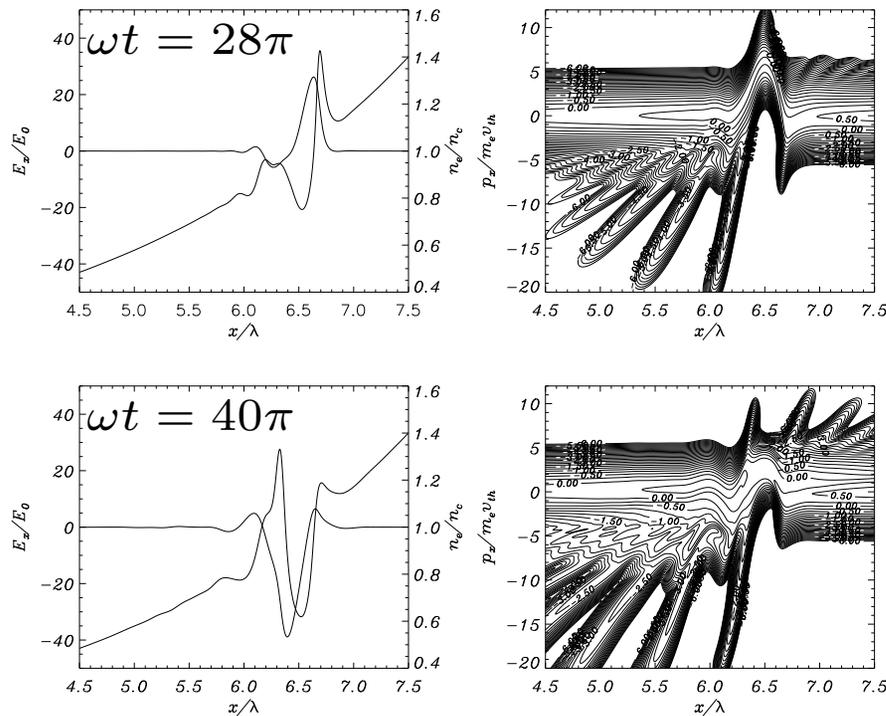
“Linear” stage: a resonantly excited plasma wave propagates towards the low density or “underdense” region ( $\omega_p < \omega$ ) region. Electrons are accelerated by the wave field.
