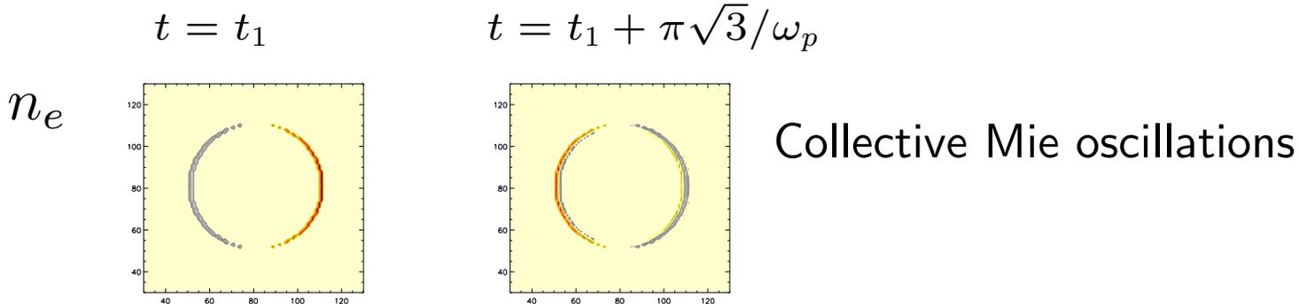
In *nanoshells* the resonance frequency depends on the shell thickness and can be tuned (applications in medicine).
