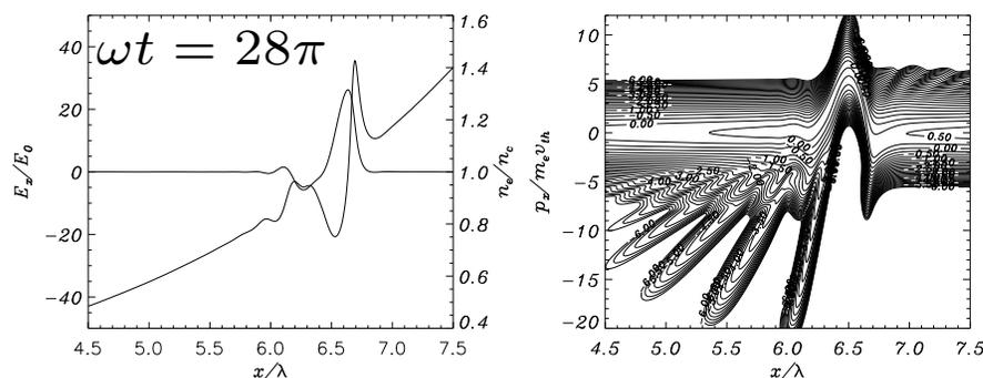
“Linear” stage: a resonantly excited plasma wave propagates towards the low density or “underdense” region ( $\omega_p < \omega$ ) region. Electrons are accelerated by the wave field.
