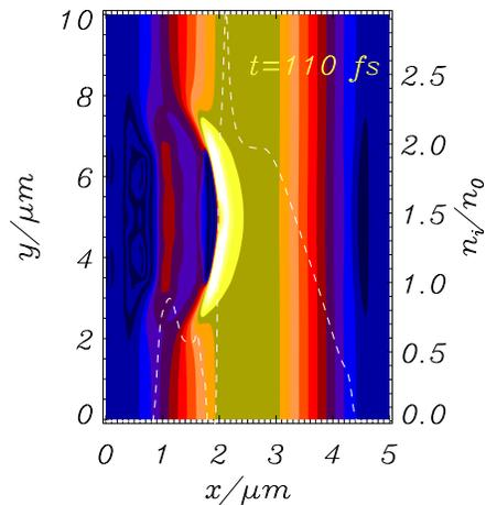
The radiation pressure modifies the plasma profile (hole boring).
