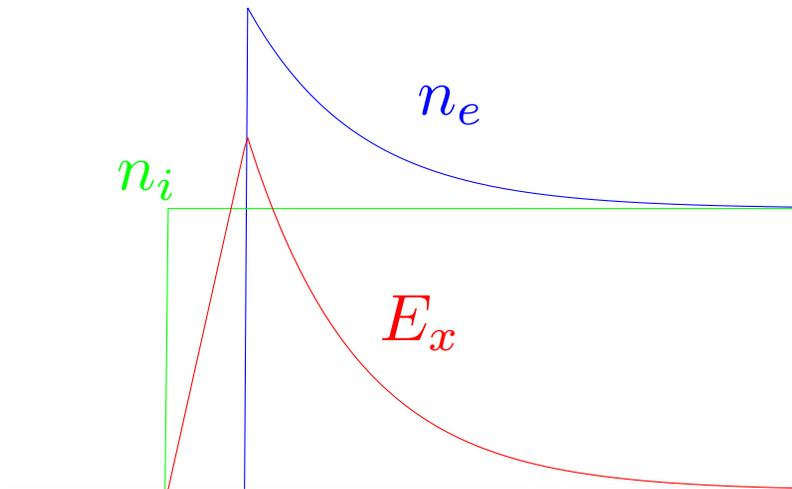
Ions will pile up forming a so-called “shock” front.
