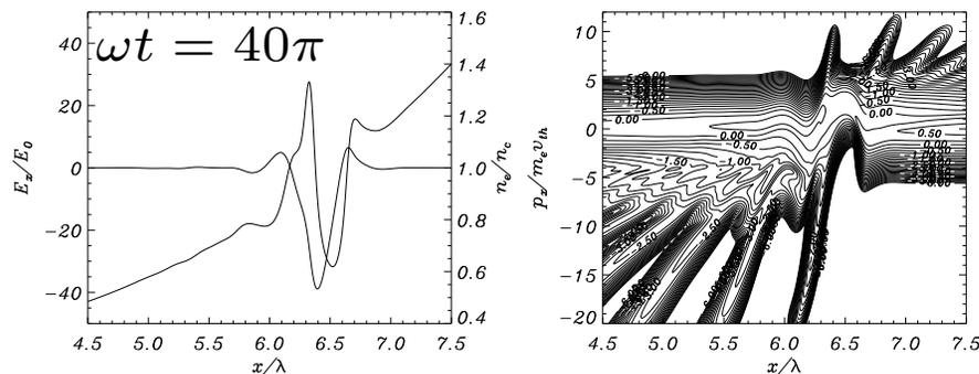
“Nonlinear” stage: the plasma density profile is strongly modified. Additional fast electrons bunches are generated at resonance and propagate into the *overdense* plasma ( $\omega_p > \omega$ ).
