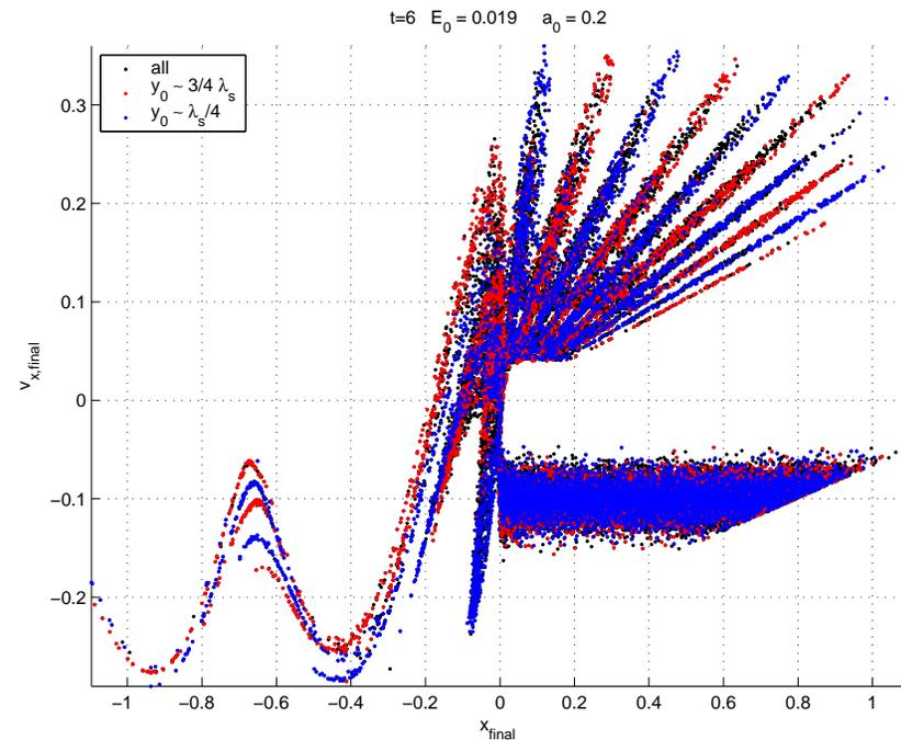
– “Jets” are produced at  $2\omega$  rate (by  $\mathbf{v} \times \mathbf{B}$  force).
