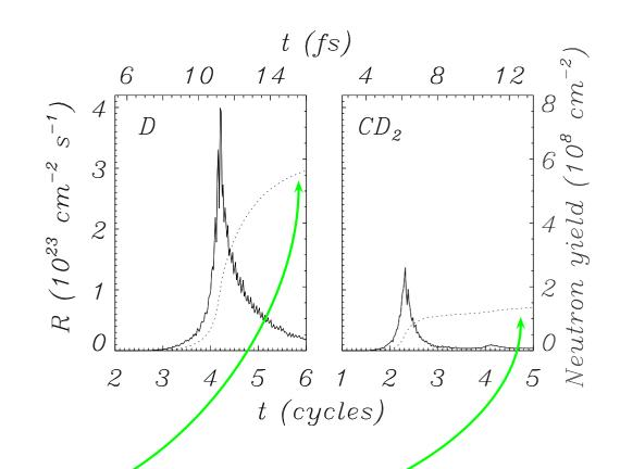
Neutron yield:  $\sim 10^3 \text{ J}^{-1} \text{ (D)}, \sim 10^2 \text{ J}^{-1} \text{ (CD}_2)$
