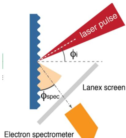
Imaging of **electrons** emitted from the front side of the target: evidence of **narrow-angle**, **intense** beam near the target surface for **grating** targets
