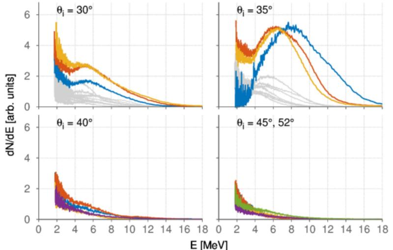
Spectrum variability (**gray** lines) related to beam direction fluctuations due to the small acceptance angle of the spectrometer
