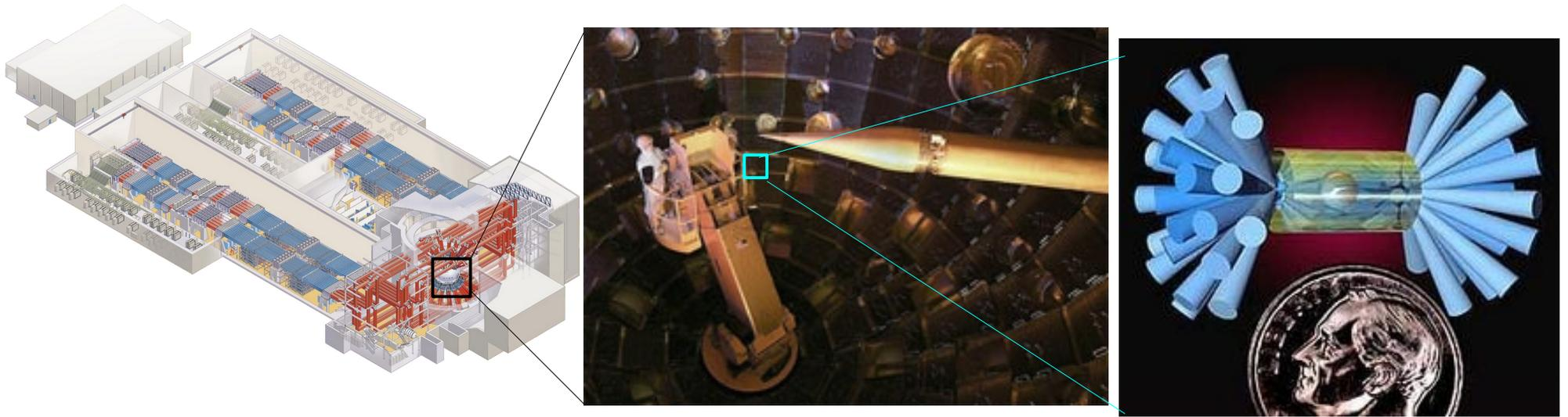
The National Ignition Facility (NIF): 192 beams focused on a DT capsule delivering up to 2 MJ at 500 TW power in few ns
