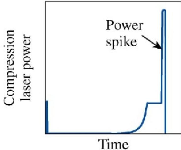
A laser pulse with a high power spike generates a strong converging shock wave which collides with the return shock; appropriate timing produces high compression in the central region (hot spot)
