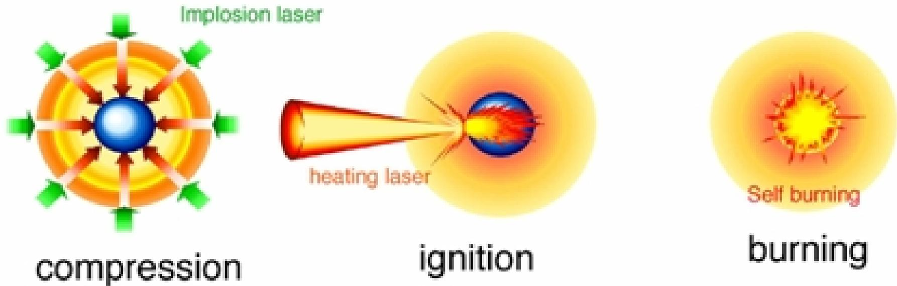
Compression is separated from ignition: a picosecond duration, petawatt power beam (either a laser pulse interaction directly with the fuel or a laser-driven proton beam externally generated) creates a “spark” to ignite the fuel and start burn in isochoric conditions
