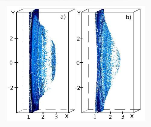
Supergaussian "flat-top" profiles keep a "quasi-1D" geometry and prevent early breakthrough of laser pulse due to lateral expansion
