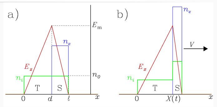
Sail (S): ions are bunched accelerated by  $E_x = f_p / e$  and move coherently as a "foil": monoenergetic component
