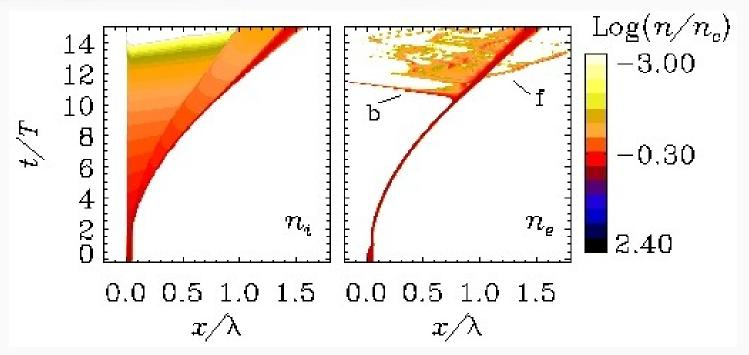
Near the end of the acceleration stage the pressure balance for electrons breaks down: formation of bunches in forward & backward directions and heating
