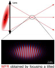
WFR obtained by focusing a tilted wavefront pulse
