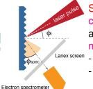
Sinusoidal gratings at SP resonance: collimated ( $\delta \phi \simeq 20^{\circ}$ ) electron emission along the surface ( $\phi \simeq 2^{\circ}$ ) multi-MeV energy, total charge  $\simeq 100$  pC
