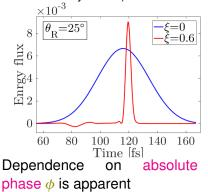
$E = E(r, z, t) \exp(-i\omega_L t + ir\zeta t + \phi)$   $\zeta$ : WFR parameter A 3.8 fs (~1.4 cycles) SP is generated from a 30 fs,  $\lambda_L = 0.8 \ \mu m$  laser pulse
