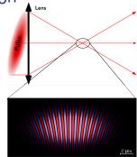
MEEP<sup>1</sup> simulations of WR pulse on Ag grating (only linear response, no nonlinear dynamics)
