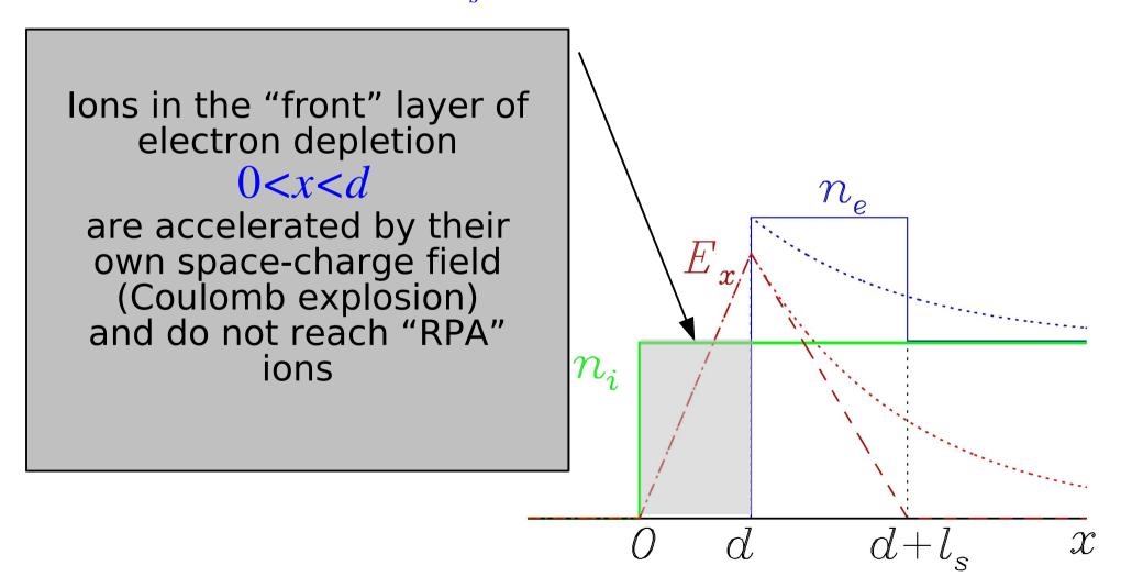
A simple modeling for RPA of semi-infinite targets ("hole boring" regime) accounts for the dynamics observed in PIC data and gives scalings for ion energy and acceleration time
