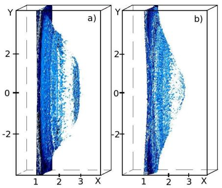
Gaussian intensity profiles lead to early "burnthough" due to lateral expansion of the target Supergaussian "flat-top" profiles, keeping a "quasi-1D geometry" are needed for efficient acceleration and to ensure high collimation and monoenergeticity
