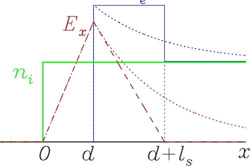
A simple modeling for RPA of semi-infinite targets ("hole boring" regime) accounts for the dynamics observed in PIC data and gives scalings for ion energy and acceleration time
