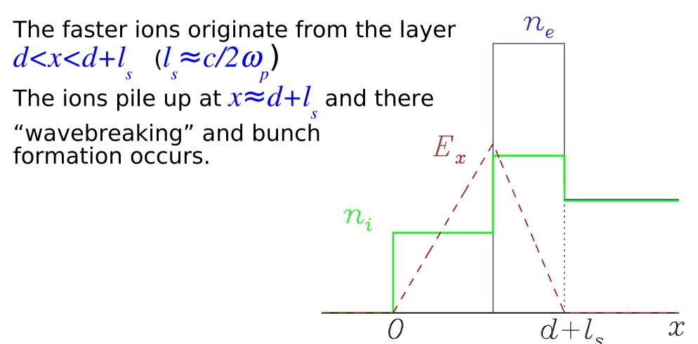
A simple modeling for RPA of semi-infinite targets ("hole boring" regime) accounts for the dynamics observed in PIC data and gives scalings for ion energy and acceleration time
