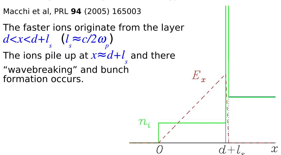
A simple modeling for RPA of semi-infinite targets ("hole boring" regime) accounts for the dynamics observed in PIC data and gives scalings for ion energy and acceleration time
