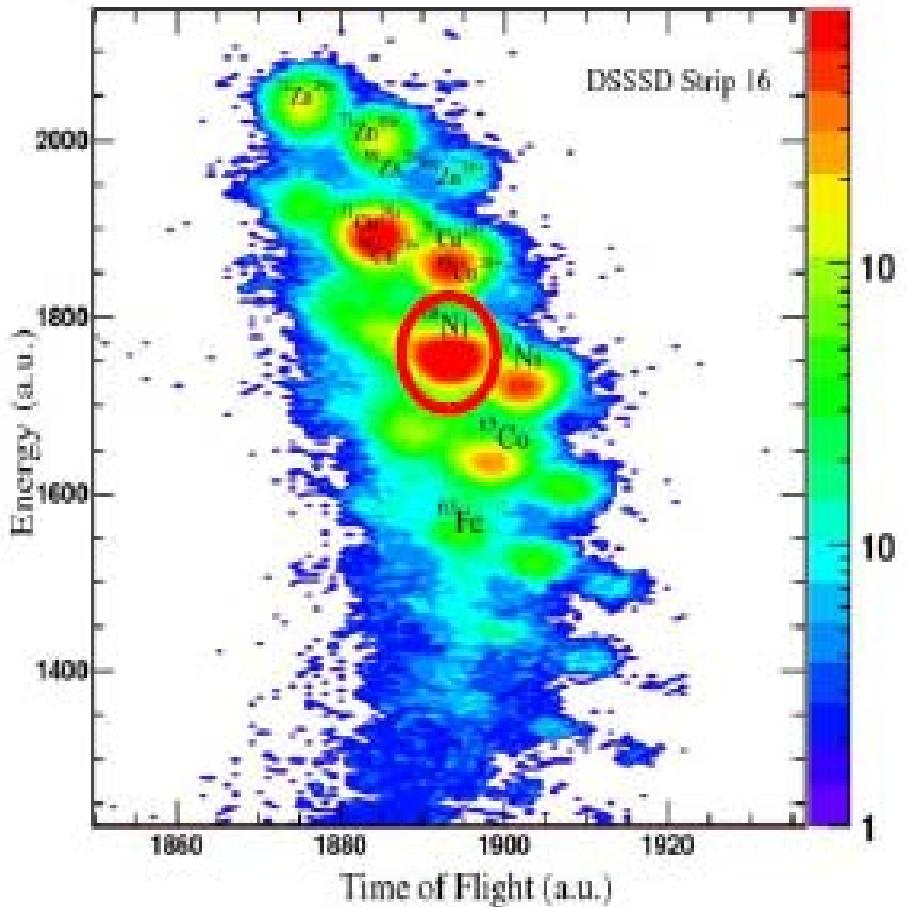
Fig.4 Identification scatter plot of  $^{68}\text{Ni}$  fragment beam
