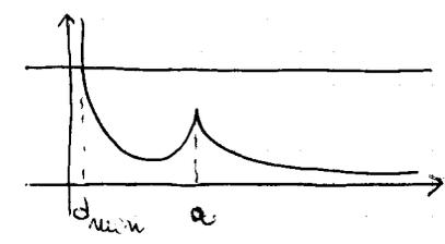
$\Rightarrow E_0 = \frac{1}{2} \mu \dot{r}^2 + \frac{L^2}{2\mu r^2} + \frac{1}{2} k_2 r^2 - \frac{1}{2} k_2 a^2 + \frac{k_1}{2a^2} \Rightarrow \tilde{E} = E_0 + \frac{1}{2} k_2 a^2 - \frac{1}{2} \frac{k_1}{a^2} =$
