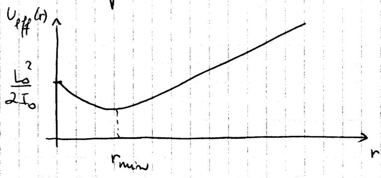
Nota circ. unif.  $\Rightarrow E = U_{\text{eff}}(r_{\min})$
