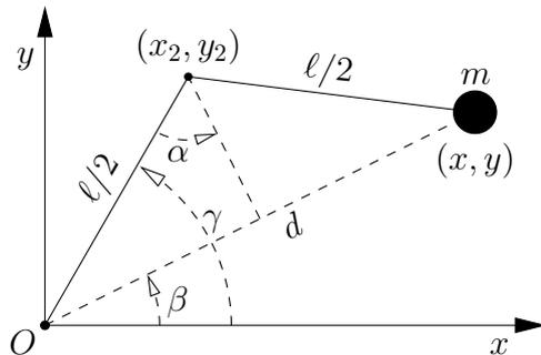
**Figure 7.5** The angles  $\alpha$ ,  $\beta$  and  $\gamma$  of Listing 7.10.
