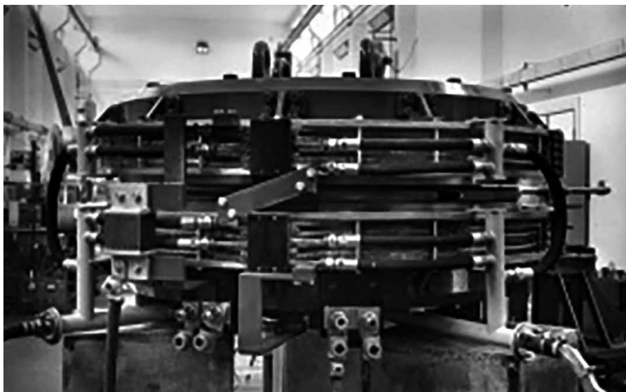
Figure 4. The storage ring AdA is shown, 1961 ( http://w3.lnf.infn.it/multimedia/ ).
