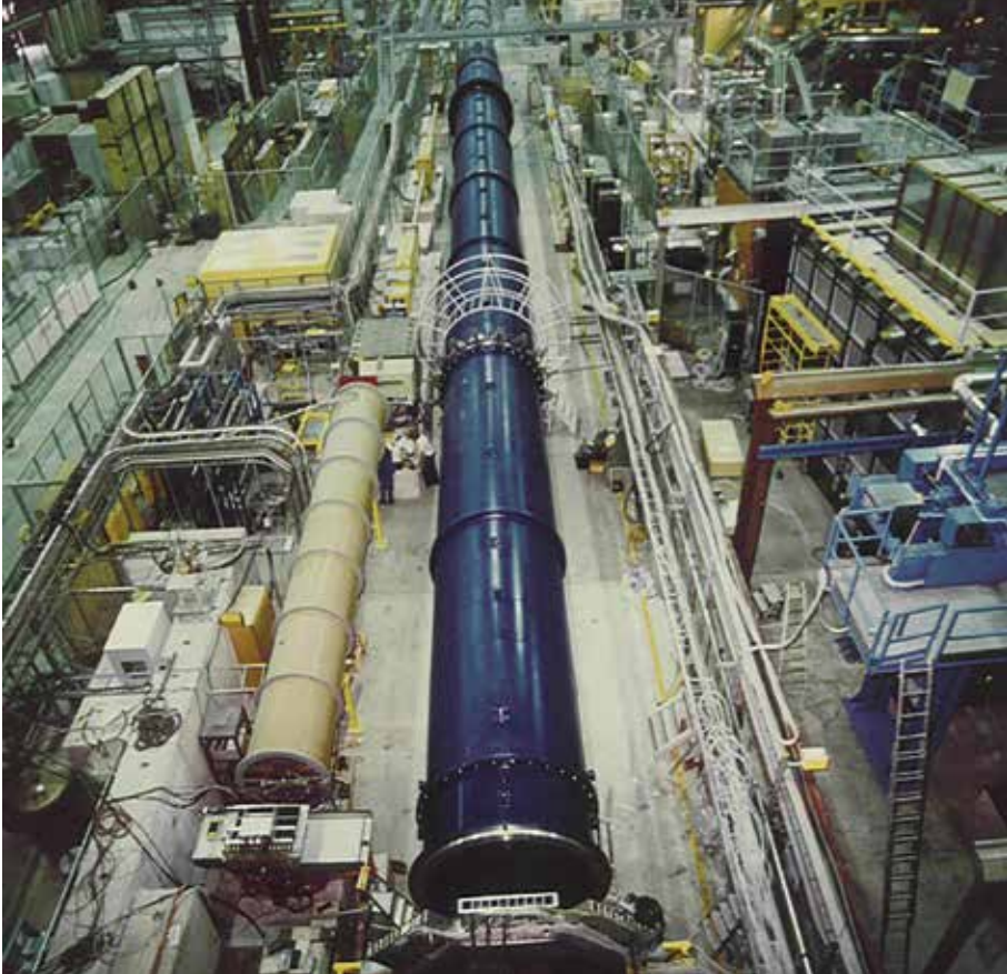
Figure 39. The K^0 decay vacuum channel of NA31 in the CERN North Area.
