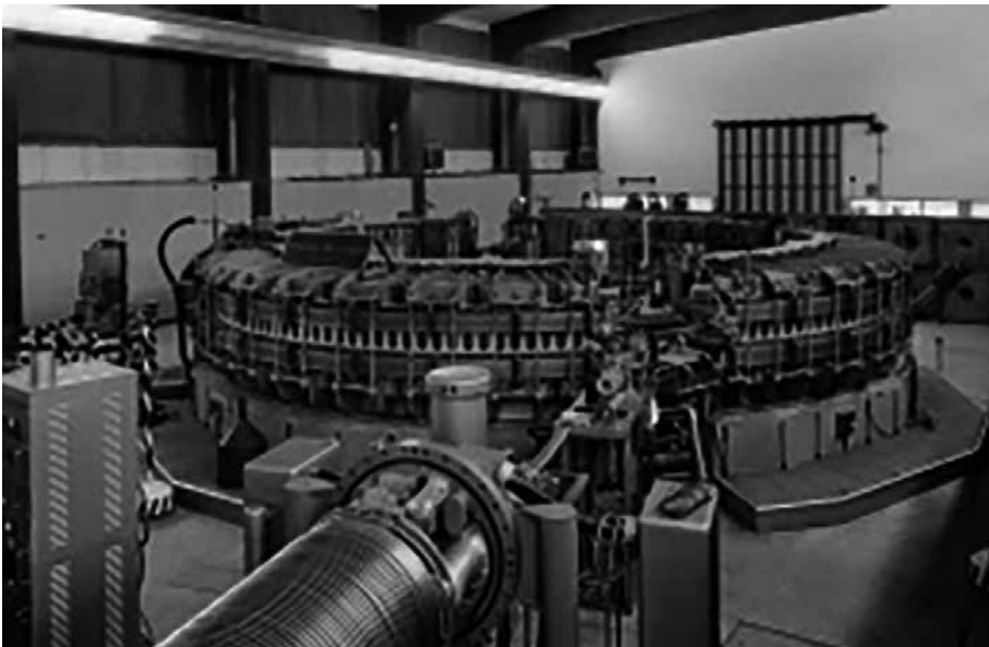
Figure 3. The electron synchrotron is displayed, 1958 ( http://w3.lnf.infn.it/multimedia/ ).
