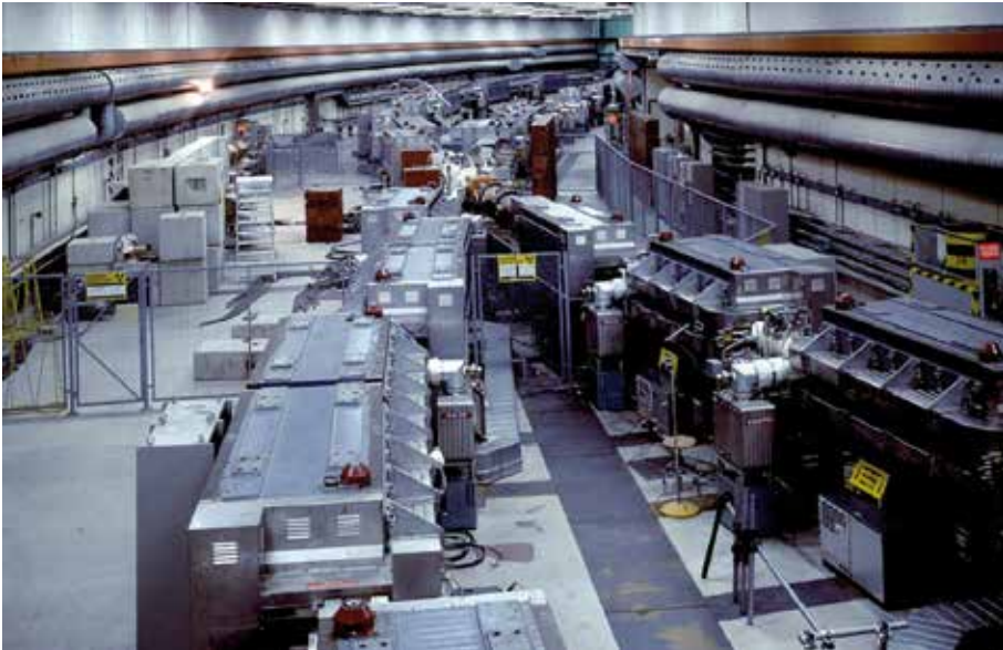
Figure 23. Picture of one of the ISR interaction region, with the two beams crossing at an angle of 15^\circ .
