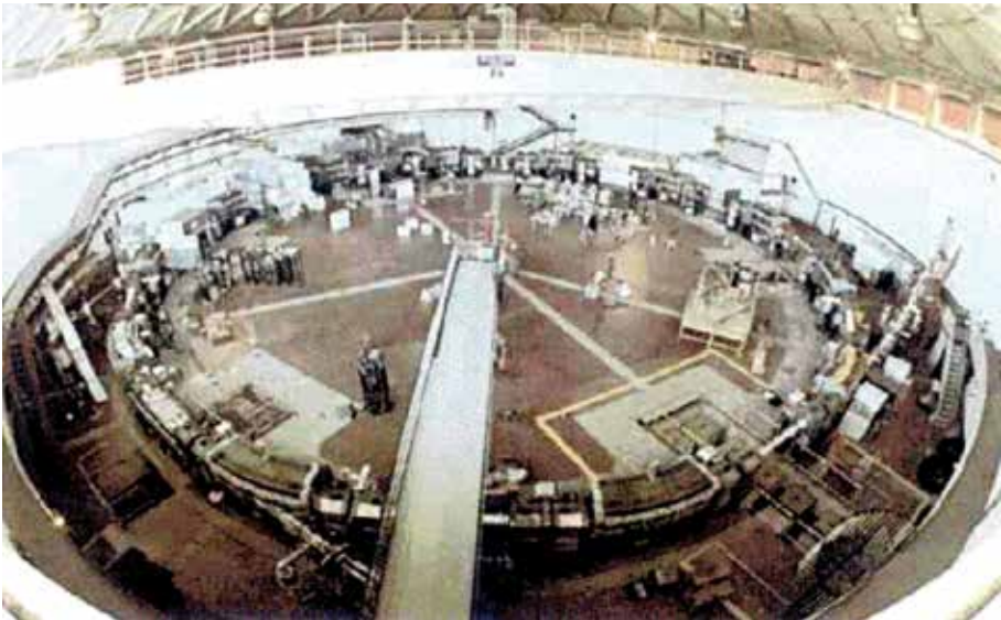
Figure 18. The 3.0 GeV e^+e^- ADONE collider.
