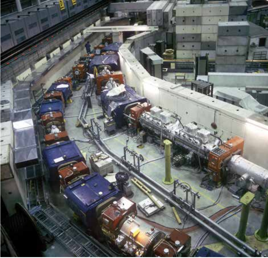
Figure 10. The CERN antiproton source after 1986: the Antiproton Collector (AC, outer ring) and the Antiproton Accumulator (AA).
