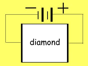
If the material, instead, is a semiconductor, such a simple approach would fail. The reason is that in a semiconductor, which has a non negligible conductivity at room temperature, the current flowing under the effect of the applied voltage and its associated noise would mask the small current signals due to the particles.
