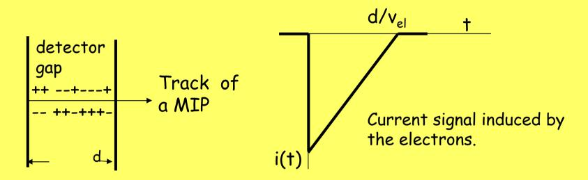
The figure on the left shows an ionization track extending across a detector gap with a uniform carrier density. The figure on the right shows the current induced on the electrode by the motion of the electrons. The positive ions are so slow that at such short times their contribution to the induced current has been neglected.
