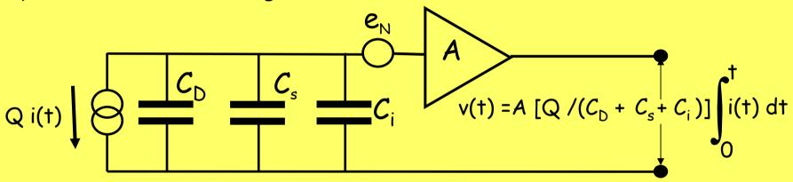
$\mathcal{C}_{s}$  represents the total stray capacitance which appears between the detector terminals
