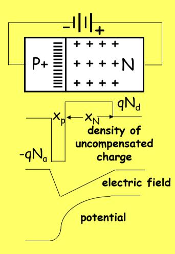
**P+region:** trivalent impurities (B) with density  $N_a$ - free carriers holes(+), ionized atoms with negative charge **N region:** penthavalent impurities (As) with density  $N_d$ , free carriers electrons (-), ionized atoms with negative charge **Charge balance:**  $x_PN_a = x_NN_d$  which shows that the space charge region extends more deeply into the region of lower impurity density. **Case of N\_a >> N\_d**, the depleted region extends almost entirely in the N region,
