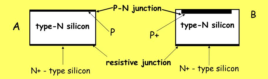
A: the junction is obtained by evaporating under vacuum a thin layer of goldB: the junction is obtained by creating a P+ layer by ion implantation
