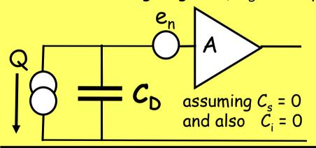
amplifier. It is understood, then, that it makes more sense to assume as a quality factor the ratio  $\varepsilon$  / dielectric constant. On this basis, diamond, which has a smaller dielectric constant, appears less unfavorable in its comparison with silicon.
