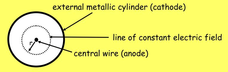
The electric field has a 1/r - dependence on the distance from the central wire. Gas multiplication is due to the accelerated electrons. It requires a sufficiently high electric field and therefore it takes place in a cylindrical layer around the central wire. Consequently it is fundamental that the central wire act as the anode.
