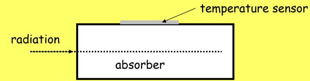
The absorber is usually made of a dielectric, diamagnetic material and operates at cryogenic temperatures, down to the mK region, to reach the highest possible temperature sensitivity by keeping the thermal capacitance as small as possible. Provided that these conditions are met, a high degree of freedom exists in the choice of the absorber material.
