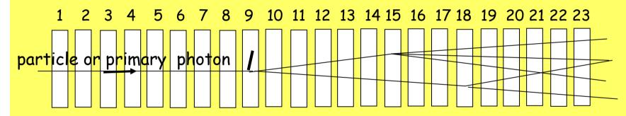
In its first implementation the active target was a telescope of silicon detectors which implemented a twofold function. Besides providing the target material it sampled the specific energy loss dE/dx in the beam direction. In its first version the active target of FRAMM experiment at CERN employed 40 silicon layers.
