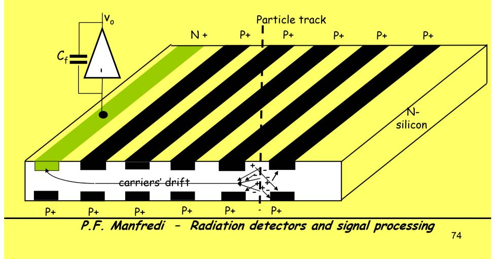
**THE DRIFT CHAMBER** - The drift chamber invented by E. Gatti and P. Rehak employs an original charge transport method. The capacitance presented to the readout preamplifier by the collecting electrode is largely independent of the sensitive area. This feature reduces the effect of preamplifier noise to a remarkable extent.
