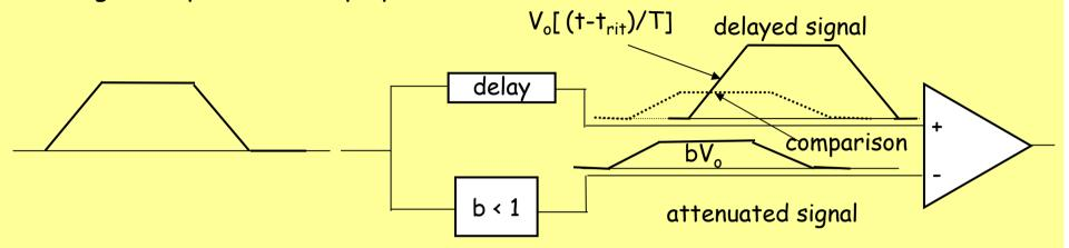
The same principle can be based upon a zero-crossing approach, as shown below
