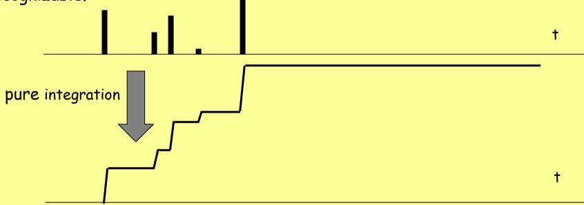
So, the first function to be implemented is some kind of differentiation (clipping) at the preamplifier output to restore the features of the individual signals.
