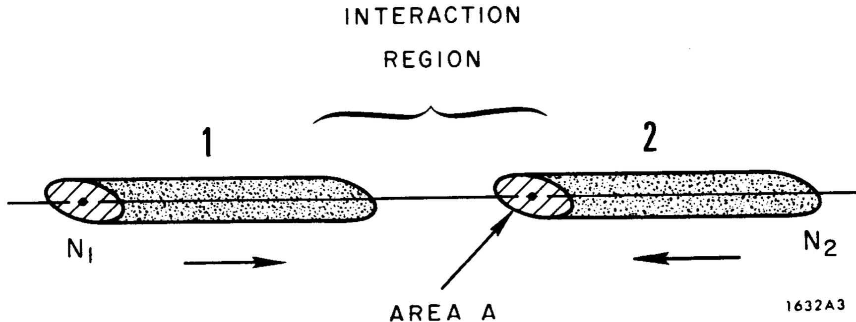
FIG. 3--Head-on collision of two bunches.
