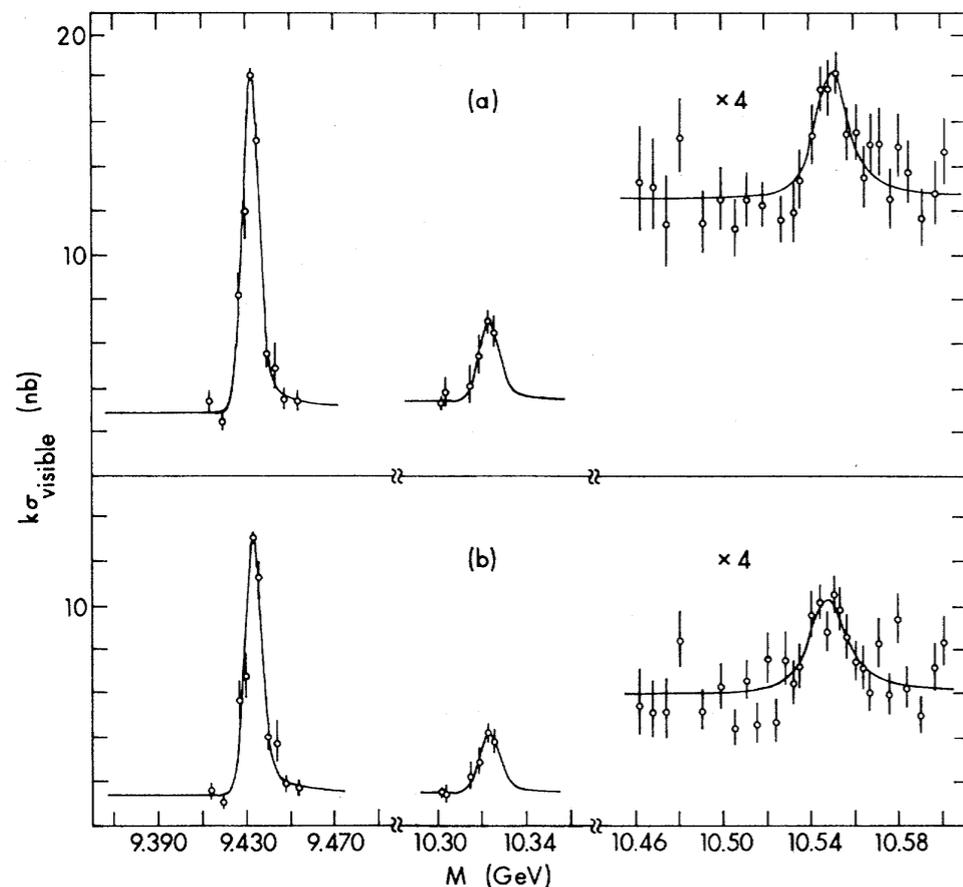
FIG. 2. (a) The observed cross section for  $e^+e^- \rightarrow \text{hadrons}$  multiplied by  $k = (M/M_\gamma)^2$ .  $M$  is the  $e^+e^-$  invariant mass. (b) The same cross section after removing events with  $T \geq 0.85$ . The lines are fitted to the data including machine energy spread and radiative corrections. See text for explanation.
