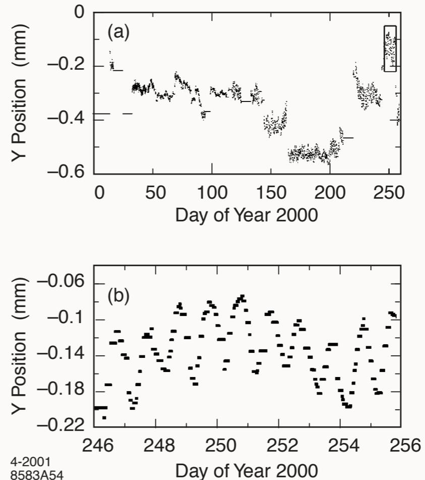
Figure 25. Global alignment of the SVT relative to the DCH based on  $e^+e^-$  and  $\mu^+\mu^-$  events: changes in the relative vertical placement measured a) over the entire ten-month run in the year 2000, and b) a ten-day period, illustrating diurnal variations.
