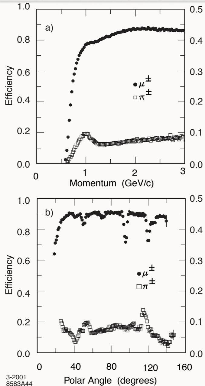
Figure 79. Muon efficiency (left scale) and pion misidentification probability (right scale) as a function of a) the laboratory track momentum, and b) the polar angle (for  $1.5 < p < 3.0$  GeV/c momentum), obtained with loose selection criteria.
