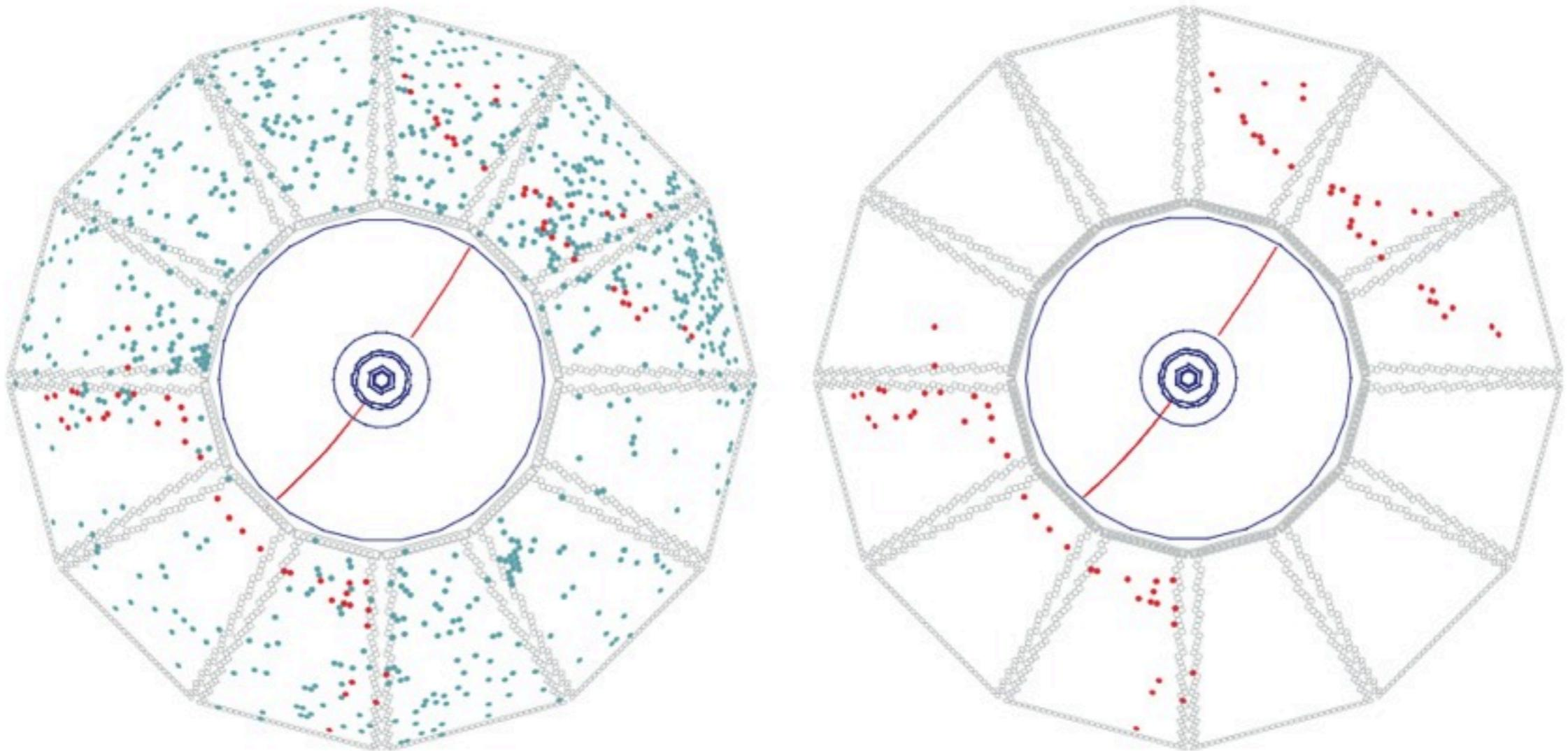
Figure 54. Display of an  $e^+e^- \rightarrow \mu^+\mu^-$  event reconstructed in *BABAR* with two different time cuts. On the left, all DIRC PMTs with signals within the  $\pm 300$  ns trigger window are shown. On the right, only those PMTs with signals within 8 ns of the expected Cherenkov photon arrival time are displayed.
