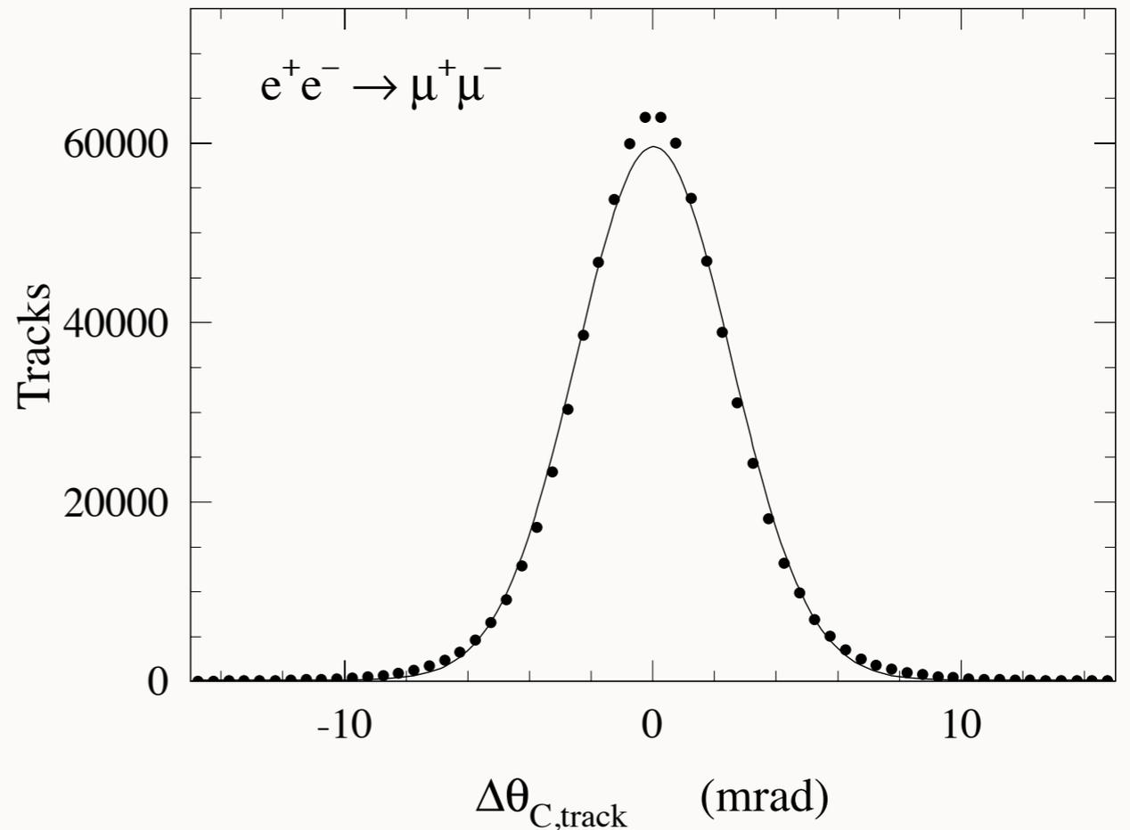
Figure 57. The difference between the measured and expected Cherenkov angle,  $\Delta\theta_{c,track}$ , for single muons in  $\mu^+\mu^-$  events. The curve represents a Gaussian distribution fit to the data with a width of 2.5 mrad.
