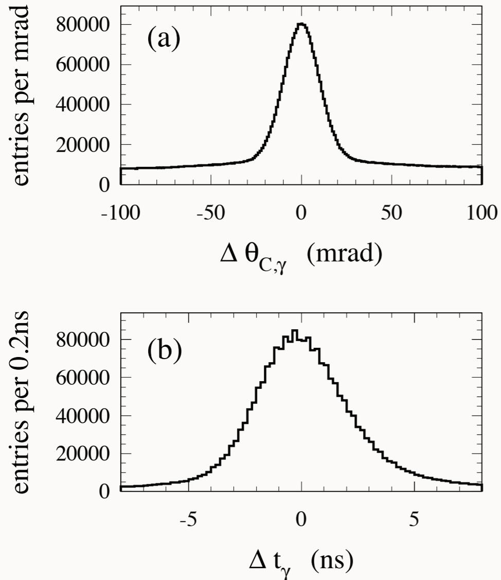
Figure 55. The difference between (a) the measured and expected Cherenkov angle for single photons,  $\Delta\theta_{c,\gamma}$ , and (b) the measured and expected photon arrival time, for single muons in  $\mu^+\mu^-$  events.
