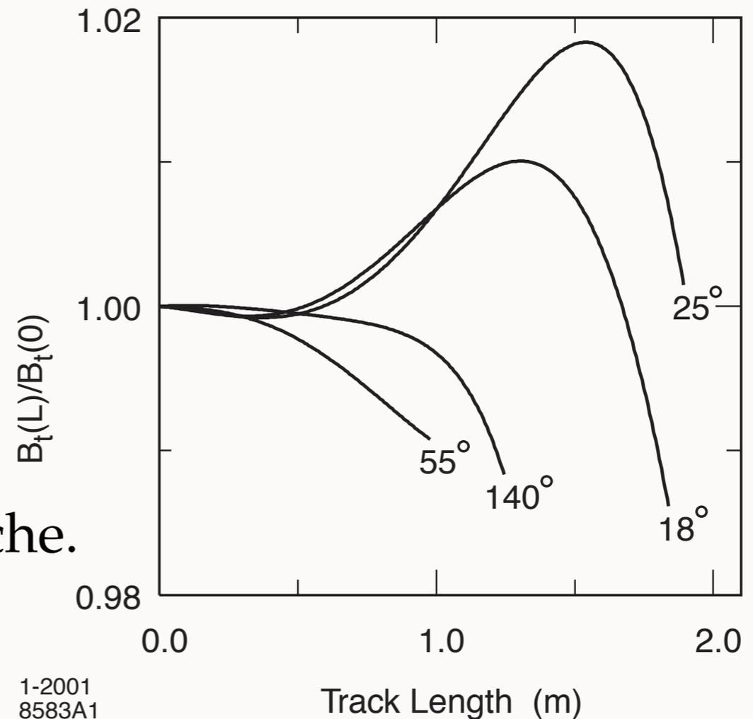
Figure 15. Relative magnitude of magnetic field transverse to a high momentum track as a function of track length from the IP for various polar angles (in degrees). The data are normalized to the field at the origin.
