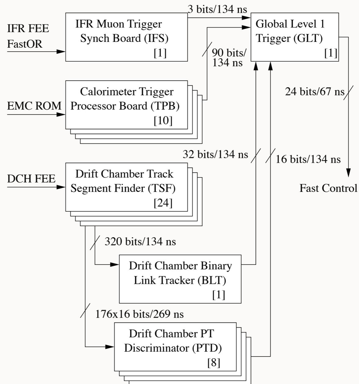
Figure 82. Simplified L1 trigger schematic. Indicated on the figure are the number of components (in square brackets), and the transmission rates between components in terms of total signal bits.
